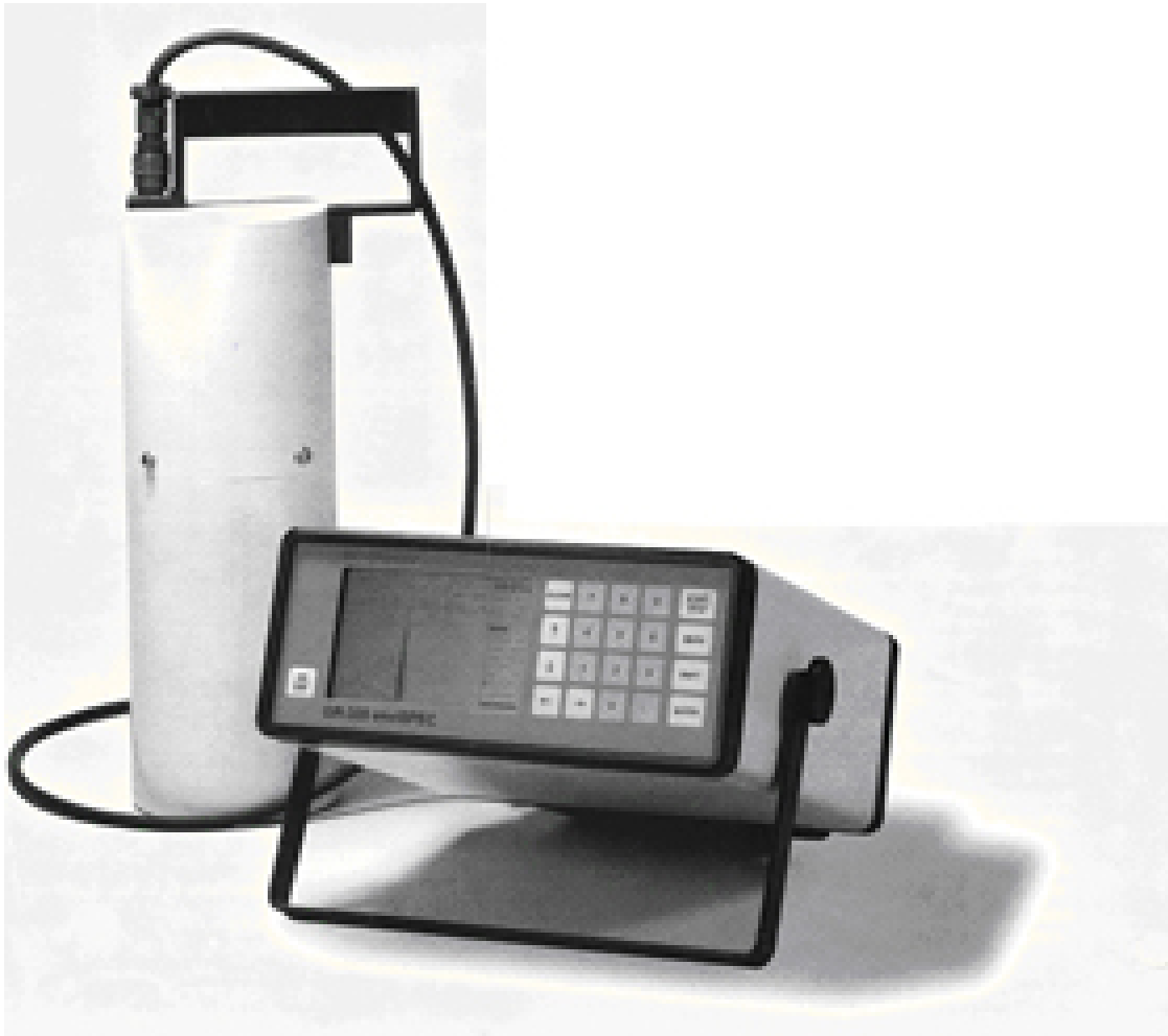
Figure 4. Photograph of the portable gamma ray spectrometer that was used to collect gamma-ray measurements from the Woodford Shale (Exploranium GR-320 Manual).
