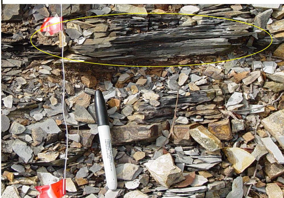
Figure 26. Woodford Shale along I-35, yellow circle indicates fissile shale that is laminated <1 cm thick.
