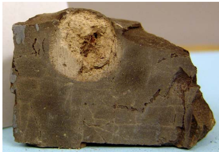
Siliceous shale sample with a phosphate nodule that was collected from the Upper Woodford shale.
