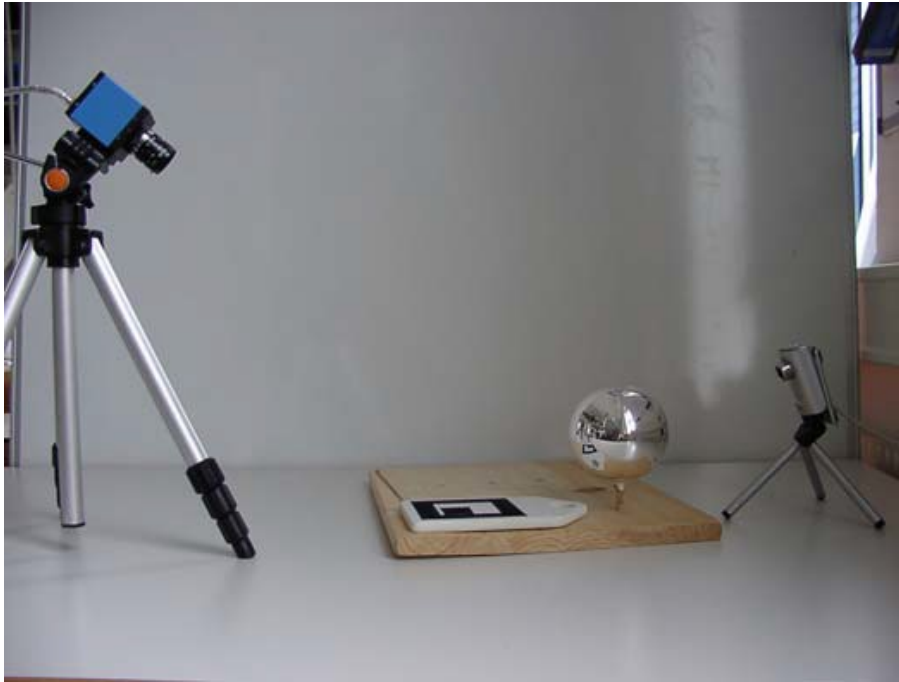
Figure 1: Configuration two of three [4]. The main viewing camera is focused on the marker (the black and white texture next to the sphere) while a second camera observes the reflection on the mirror ball
