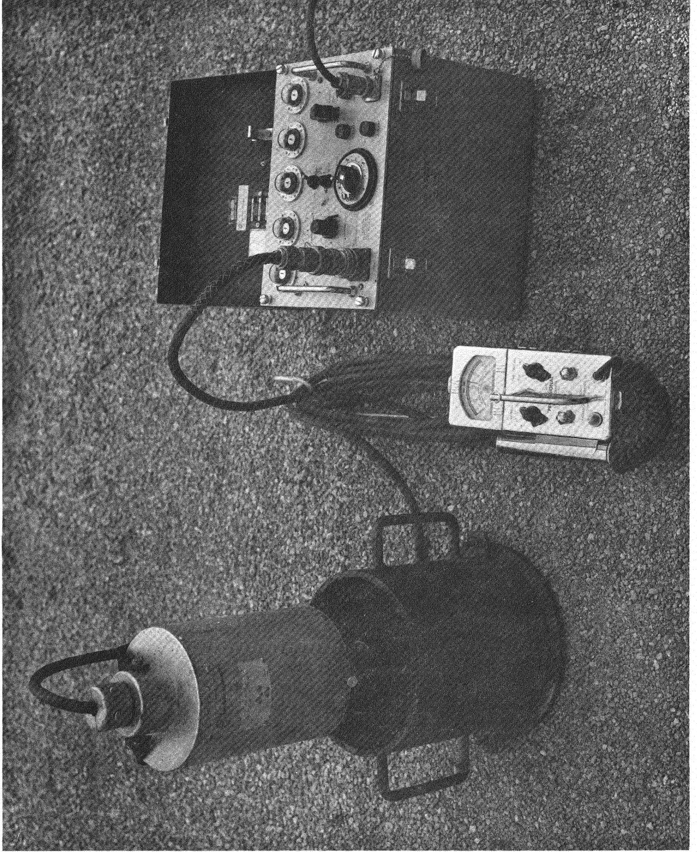
Figure 37. Field Recording setup (Sample and Nuclear Device).
