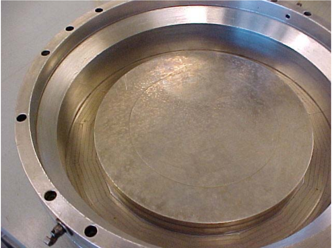
Figure 4.11 - Photograph of Chamber Base Showing Arrangement of the Magnets
