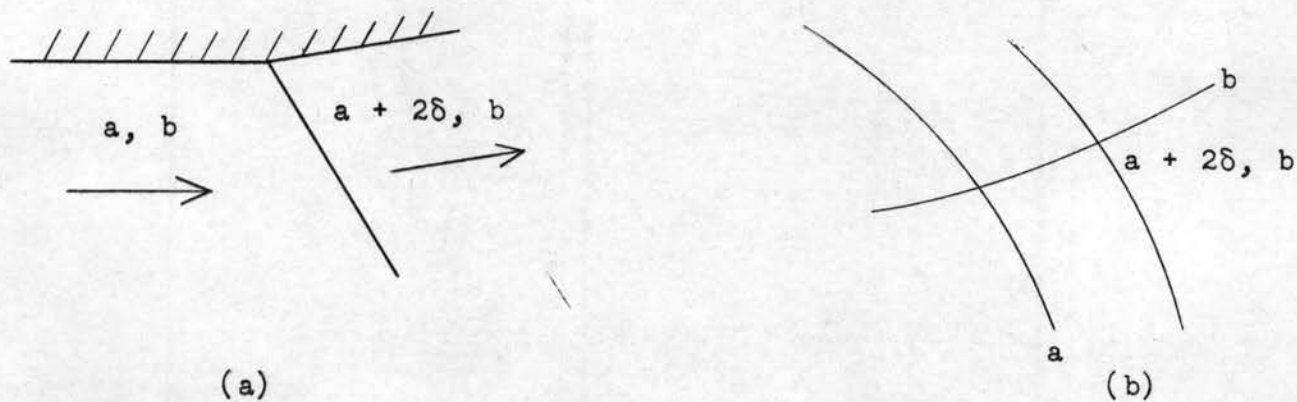
Fig. 13. Origin of Expansion Wave.
