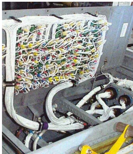
Figure 4. 1 Example of cable bundles inside aircraft cockpit
