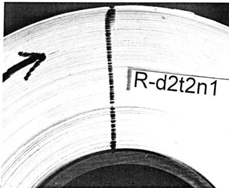
Figure 62c. Photograph of the wound roll showing slippage after the Dynamic Torque test. The Nip diameter is 6 inches and the W.O.T for the roll is 0.67 pli. The parent roll id. is 1, the diameter of the wound roll is 7.51 inches, the Half width of contact is 0.219 inches and the nip load is 0.83 pli.
