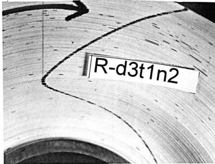
Figure 60e. Photograph of the wound roll showing slippage after the Dynamic Torque test. The Nip diameter is 8 inches and the W.O.T for the roll is 0.3 pli. The parent roll id. is 7, the diameter of the wound roll is 8.01 inches, the Half width of contact is 0.281 inches and the nip load is 5 pli.
