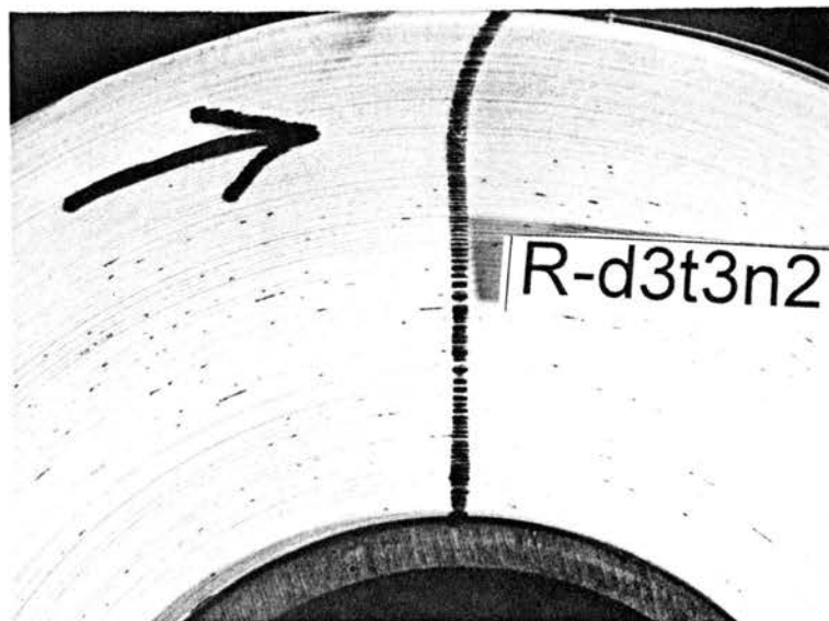
Figure 66d. Photograph of the wound roll showing slippage after the Dynamic Torque test. The Nip diameter is 8 inches and the W.O.T for the roll is 1.3 pli. The parent roll id. is 4, the diameter of the wound roll is 7.54 inches, the Half width of contact is 0.219 inches and the nip load is 5 pli.
