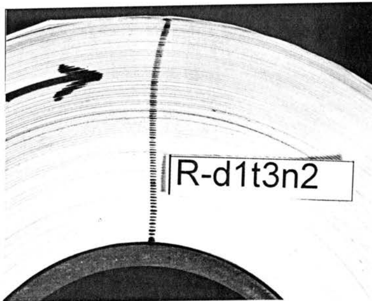
Figure 64d. Photograph of the wound roll showing slippage after the Dynamic Torque test. The Nip diameter is 2.5 inches and the W.O.T for the roll is 1.3 pli. The parent roll id. is N6, the diameter of the wound roll is 7.30 inches, the Half width of contact is 0.172 inches and the nip load is 5 pli.
