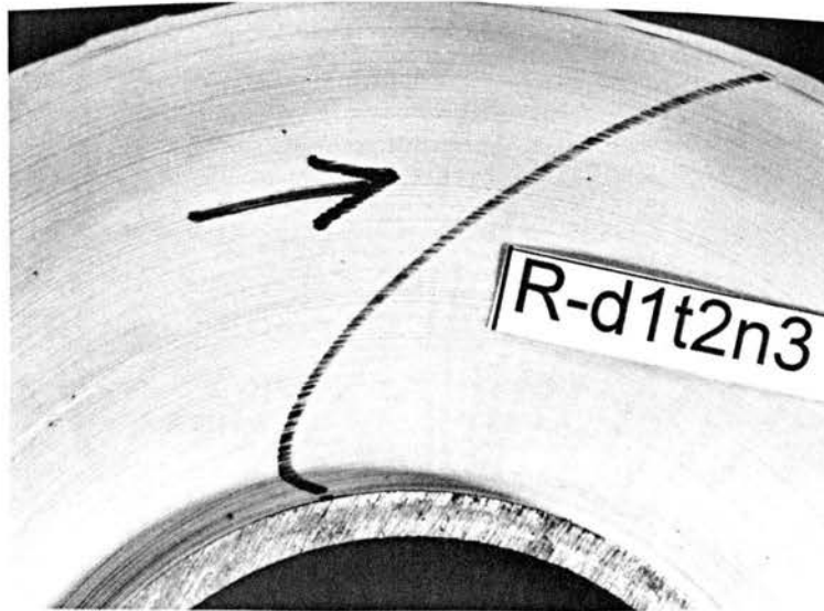
Figure 61e. Photograph of the wound roll showing slippage after the Dynamic Torque test. The Nip diameter is 2.5 inches and the W.O.T for the roll is 0.67 pli. The parent roll id. is N5, the diameter of the wound roll is 7.37 inches, the Half width of contact is 0.219 inches and the nip load is 10 pli.
