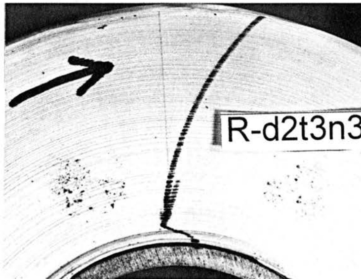
Figure 65e. Photograph of the wound roll showing slippage after the Dynamic Torque test. The Nip diameter is 6 inches and the W.O.T for the roll is 1.3 pli. The parent roll id. is N10, the diameter of the wound roll is 7.63 inches, the Half width of contact is 0.234 inches and the nip load is 10 pli.
