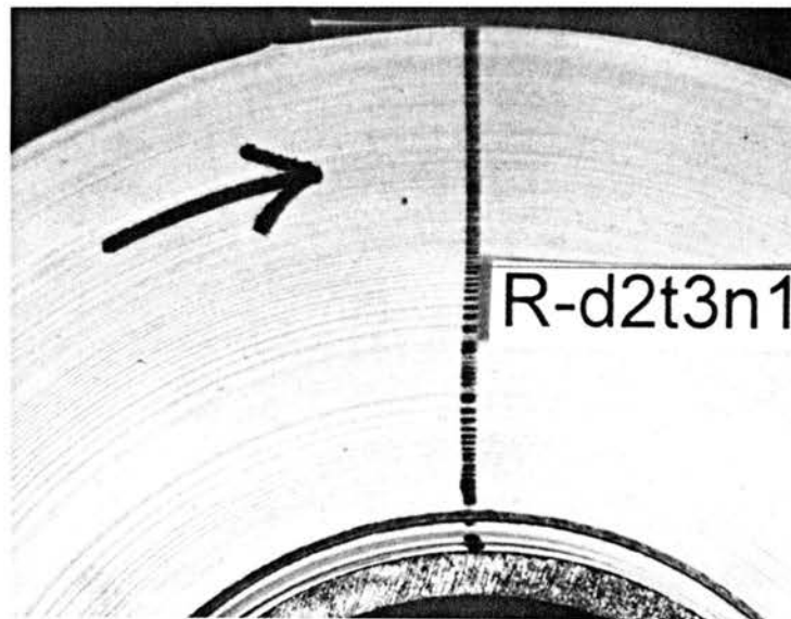
Figure 65c. Photograph of the wound roll showing slippage after the Dynamic Torque test. The Nip diameter is 6 inches and the W.O.T for the roll is 1.3 pli. The parent roll id. is N10, the diameter of the wound roll is 7.66 inches, the Half width of contact is 0.227 inches and the nip load is 0.83 pli.
