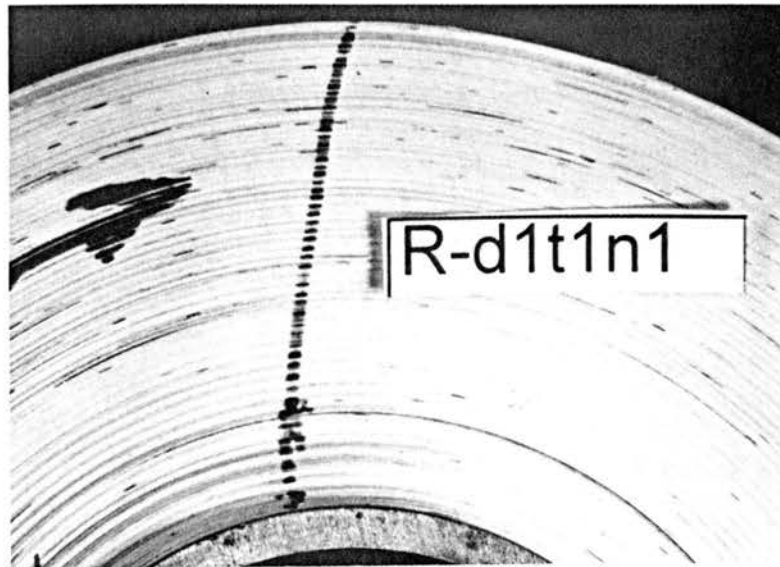
Figure 58d. Photograph of the wound roll showing slippage after the Dynamic Torque test. The Nip diameter is 2.5 inches and the W.O.T for the roll is 0.3 pli. The parent roll id. is 4, the diameter of the wound roll is 7.62 inches, the Half width of contact is 0.094 inches and the nip load is 0.83 pli.
