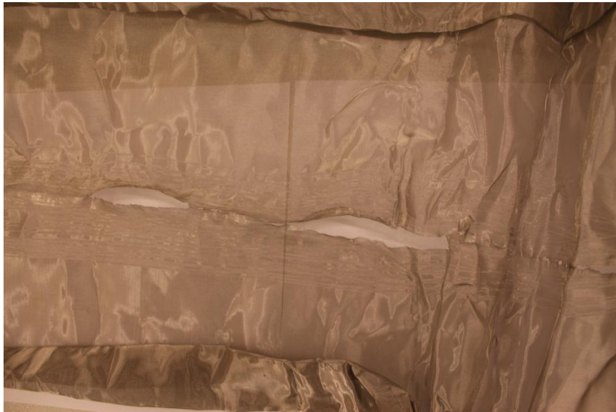
Fig 2.16 Damaged 150 x 150 (top) and 200 x 200 (bottom) Mesh Wire Cloth
