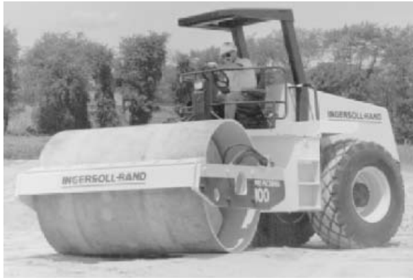
Figure 1 Vibratory roller compactor (courtesy of Ingersoll-Rand Corporation).
