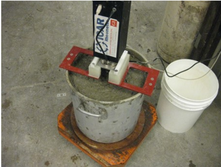
Figure 2-8: The ICAR rheometer measuring the rheology of the concrete mixture
