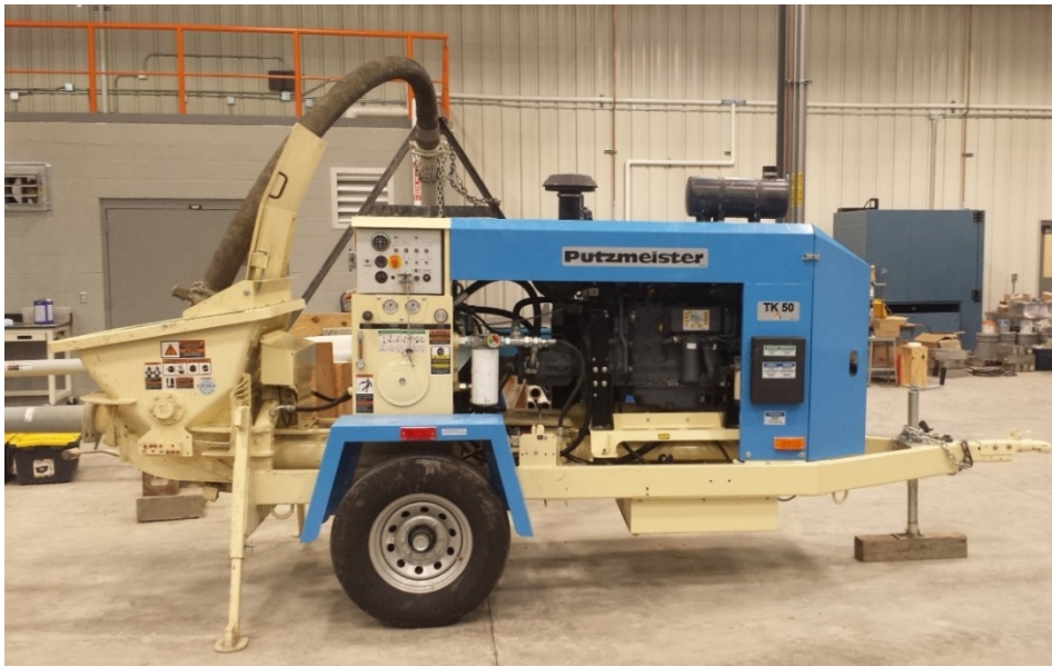
Figure 5-1: The concrete pump used in this work (Putzmeister TK 50).
