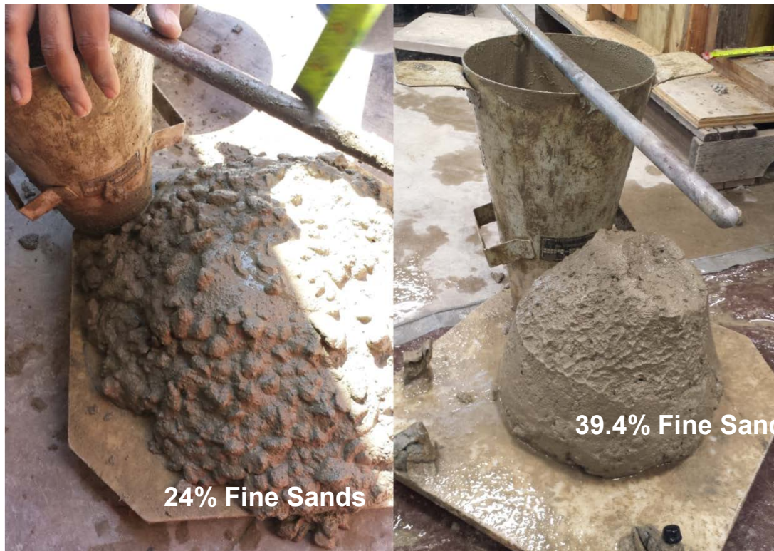
Figure 5-18 Concrete with 24% fine sands breaks apart when the Slump Test is conducted.
