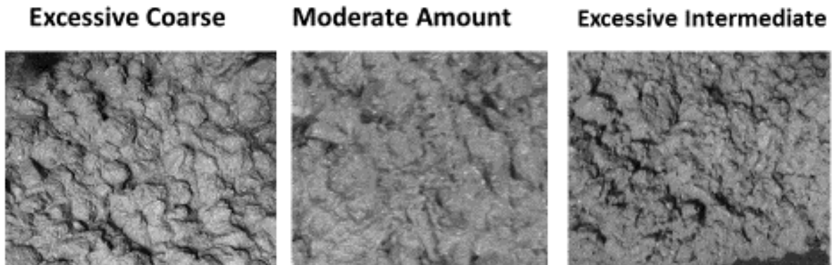
Figure 3-2: Examples of excessive amounts of coarse and intermediate sieve sizes
