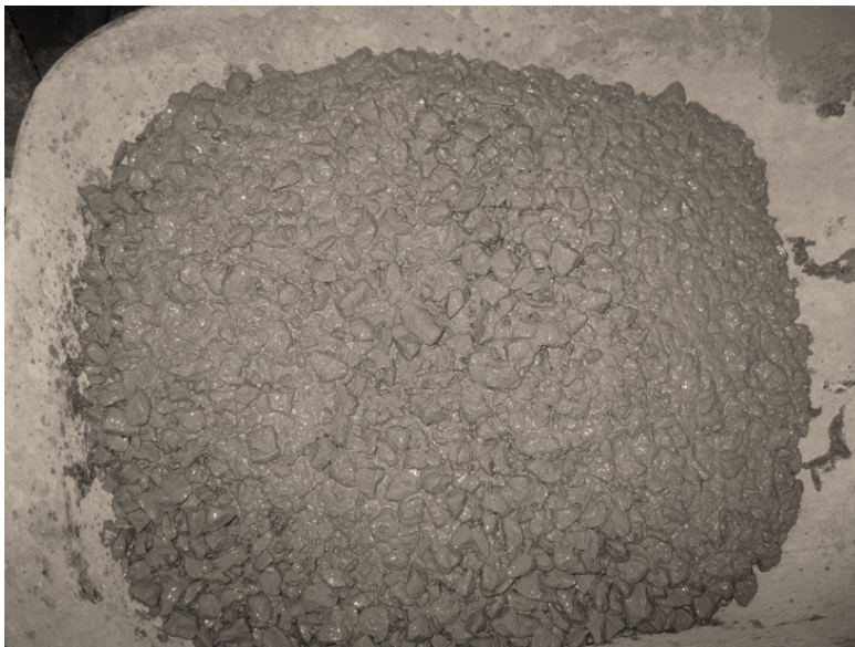
Figure 4-13: Mixture with poor cohesion of mixture 39 without #8 and #16.
