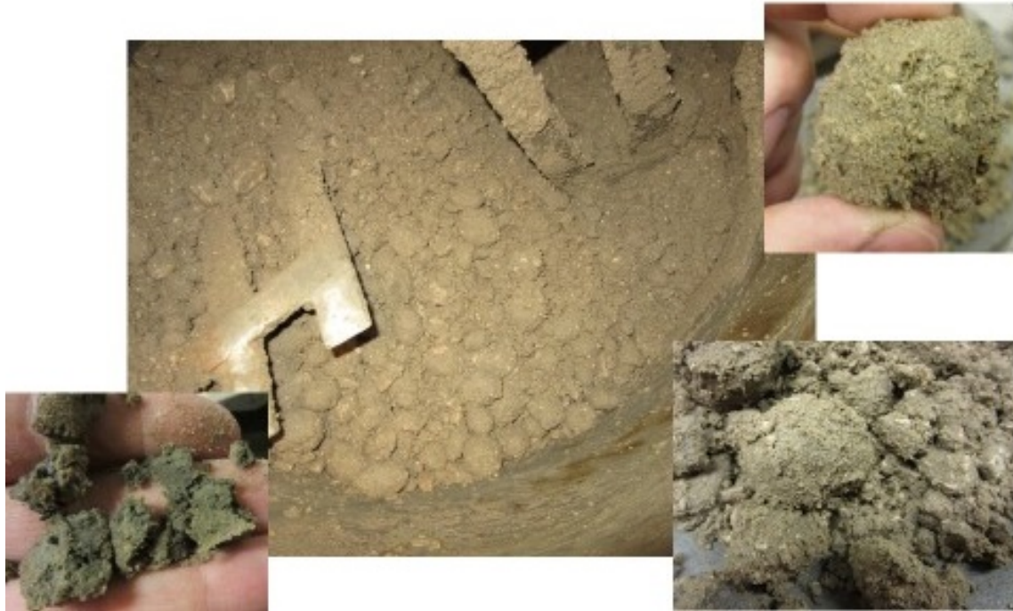
Figure 4-11: Pictures of mixtures with excessive amounts of #100 and #200 in mixture 30.
