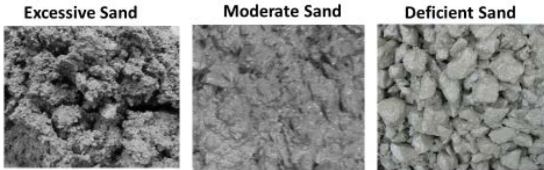
Figure 4-2: Images showing the visual observation with excessive and deficient amounts of sand
