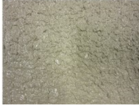
Figure 4-9: Pictures of mixtures with excessive amounts of #30 in mixture 27
