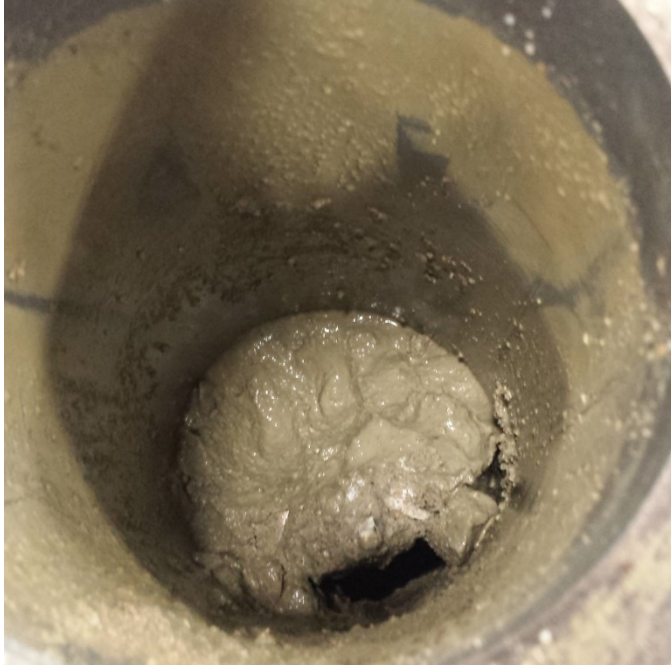
Figure 5-19: Concrete with 24% fine sands has insufficient mortar to move the aggregate, thus jamming the reducer.
