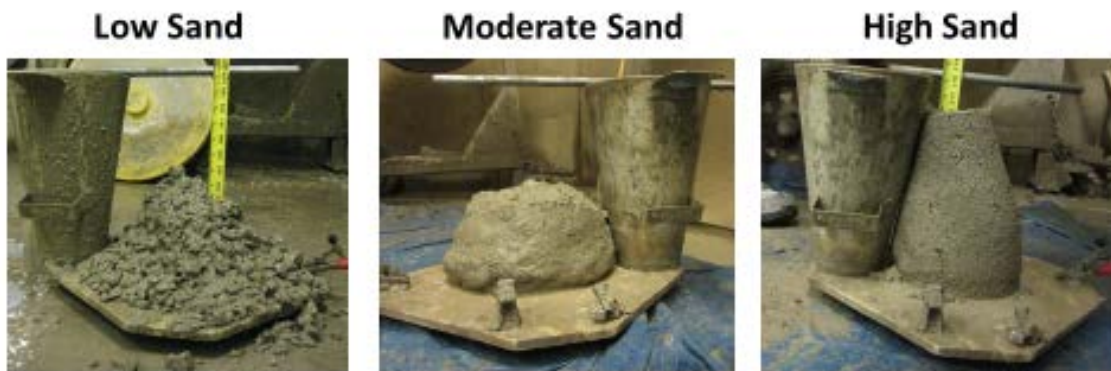
Figure 4-3: Images showing the Slump Test measuring the excessive and deficient amounts of sand.
