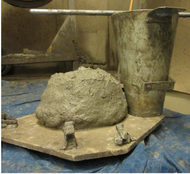
Figure 2-1: The Slump Test conducted on a structural concrete mixture.
