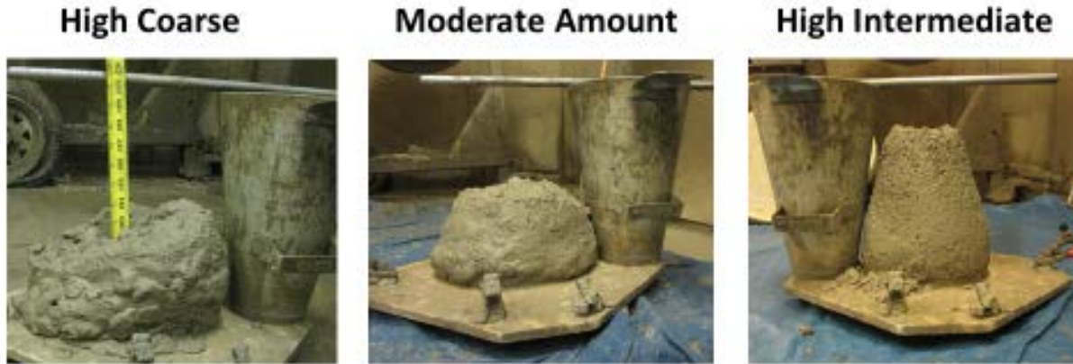
Figure 3-3: The Slump Test with excessive amounts of coarse and intermediate sieve sizes
