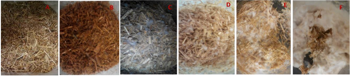
Fig. 5.3. Fungal colonization on switchgrass samples with 50% MC, 20 ml inoculum. A: raw switchgrass, B: control, C: fungal colonization at one week, D: fungal colonization at two weeks, E: fungal colonization at four weeks, F: fungal colonization at eight weeks.
