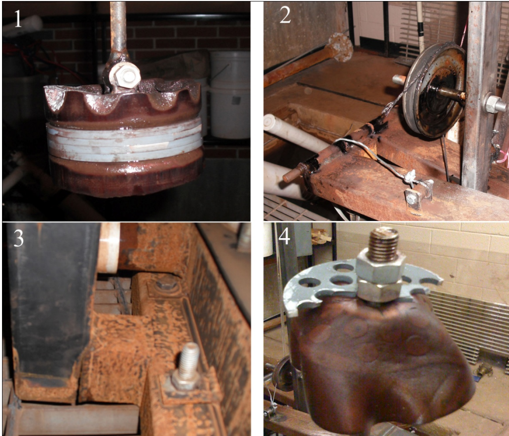
Figure 28: Broken parts: 1-treadle piston with damaged leather cups; 2- treadle pulley assembly with broken cable; 3-treadle body with broken support; 4- rower piston with broken disk.
