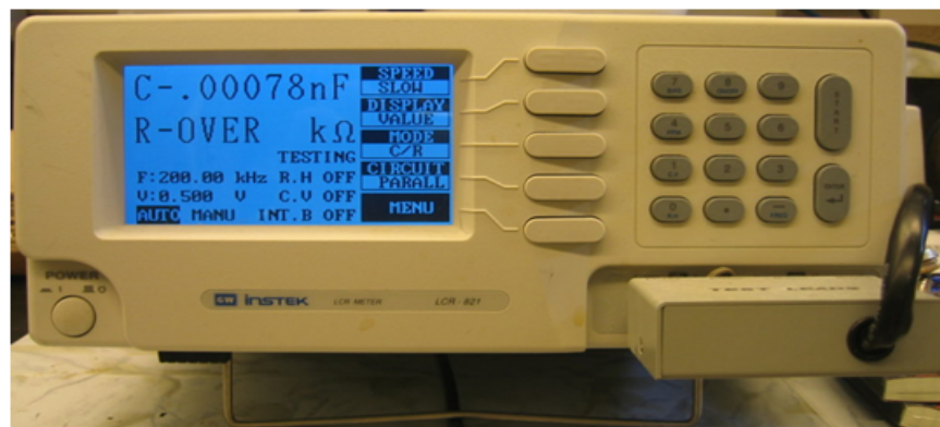
Figure 8: Instek LCR 821 high precision databridge
