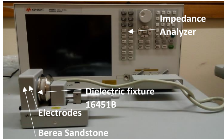
Figure A.1 Dielectric Fixture 16451B and Impedance Analyzer E4990A setup Dielectric Measurement
