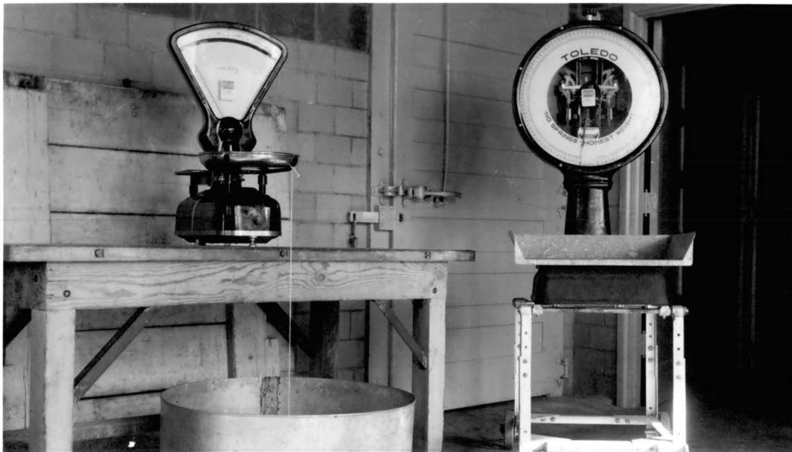
Figure 1. The equipment used in obtaining the specific gravity values of the swine carcasses.
