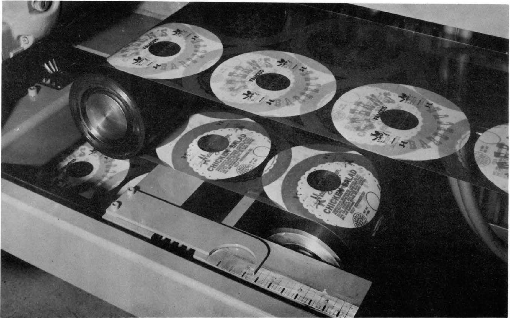
Figure 2.2.3. Drive and Tensioning Roller of Web Guiding Test Machine.
