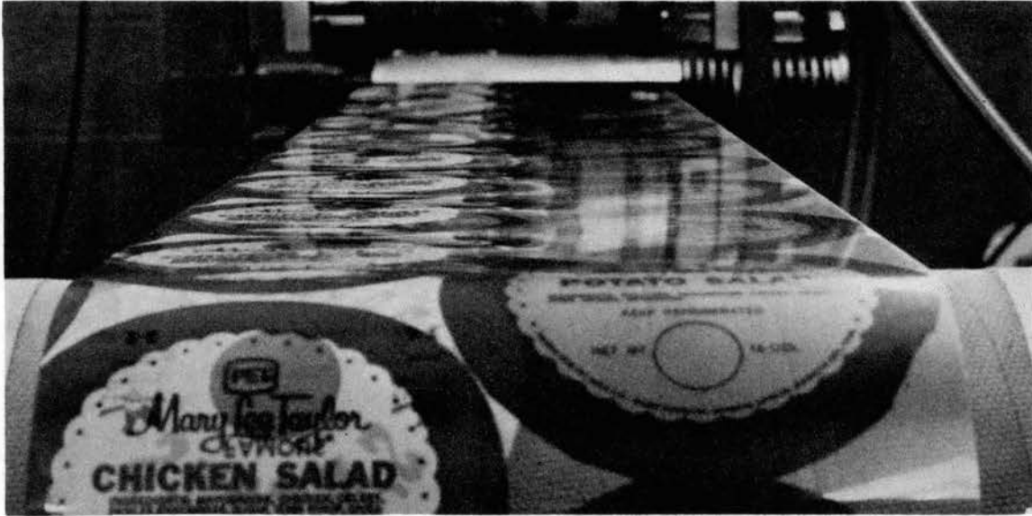
Figure 1.3.1. Web at Low Tension, With Buckles Caused by Imperfections.
