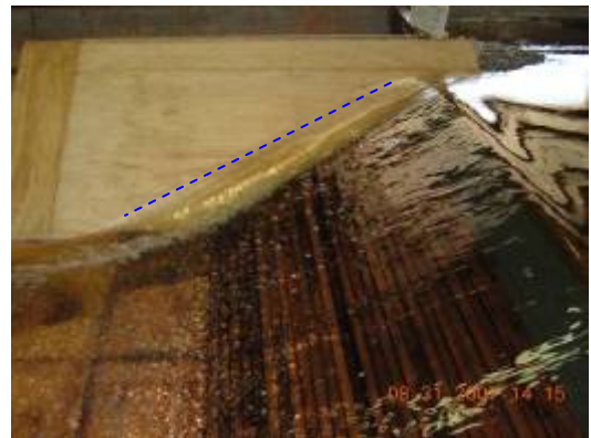
Figure 2.7. Photograph of model with 1:1 smooth training wall, d_c = 0.085 m (0.28 ft)
