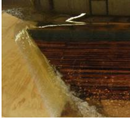
Figure 3.6. Shockwave along the training wall due to convergence on a 2:1 smooth sloped training wall.
