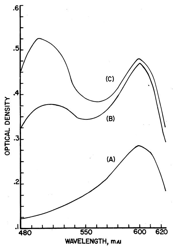
products formed from incubation of cell-free extracts with ribose 5-phosphate and co-factors for 10 minutes and 120 . minutes, respectively. The peak near 505 mu is evidence for the formation of heptulose (Dische, Shettles, and Osnos, 1949). This procedure does not distinguish between gluco-, manno-, and sedoheptulose. The increase in optical density at 600 mu indicates an increase in hexose.
