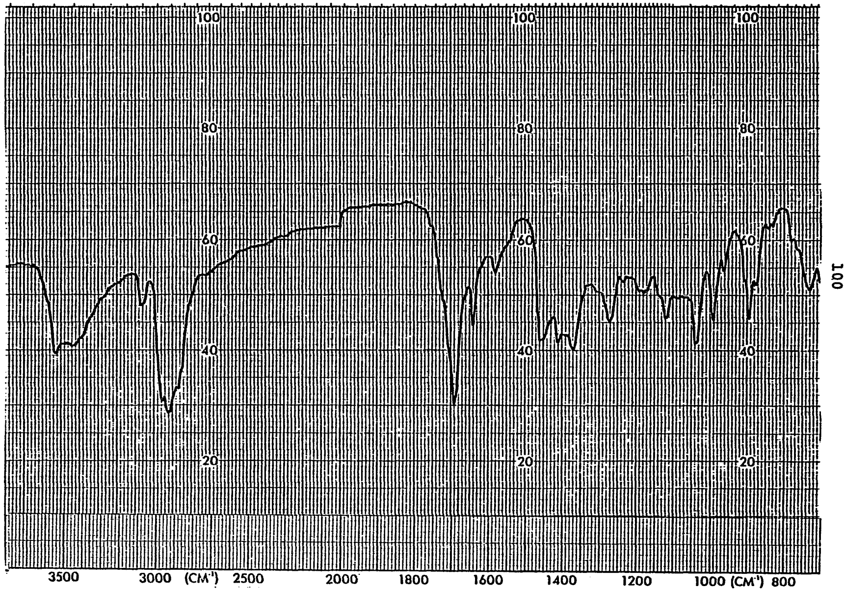
Figure 30. The ir spectrum of fraction II (diterpenoid II) isolated from Plexaura REM , St. Croix.
