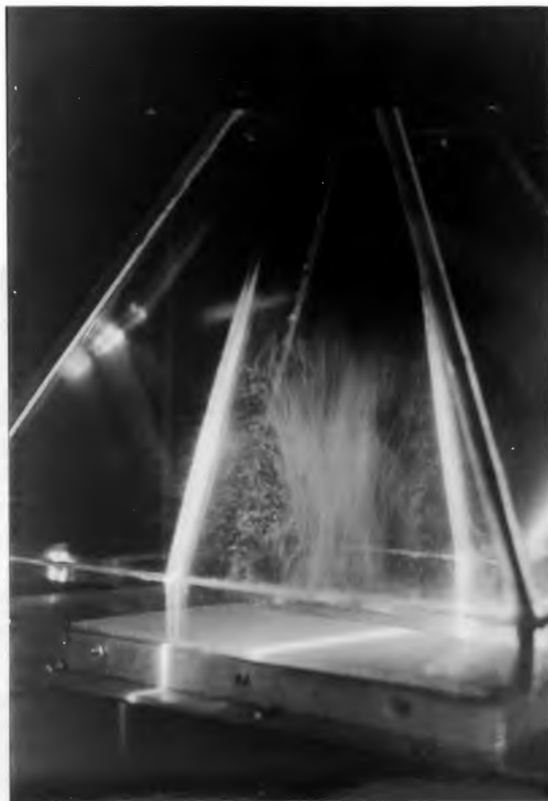
Figure 4.1 Axial Laser Sheet Water Droplet Flow Visualization within the SAE Test Housing (Sabnis, 1993).
