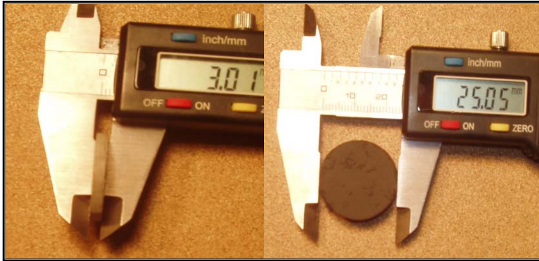
Figure (5-1): Disk sample (25 mm diameter and 3 mm thick) for osmotic and permeability test.
