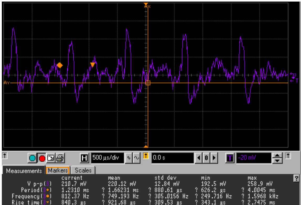
Figure 4.15 Output pulse signal when sensed pulsed input equals 200uV @ 1kHz in saline solution
