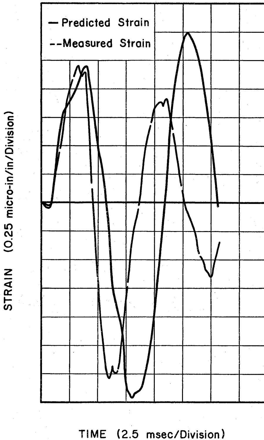
Figure 22. Comparison of Predicted Strain Response to Measured Strain for Center of Panel in Baffle, P = 0.2 psf N-wave, \tau = 0.00672 sec
