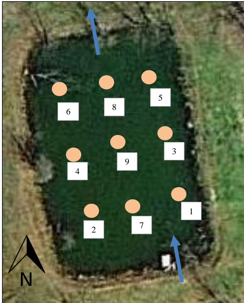
Figure 2-5 Diagram of the nested piezometer at the Red Oak PTS. Locations are approximate. The blue arrows indicate where the water enters and leaves the cell. (Google Earth B 2013)
