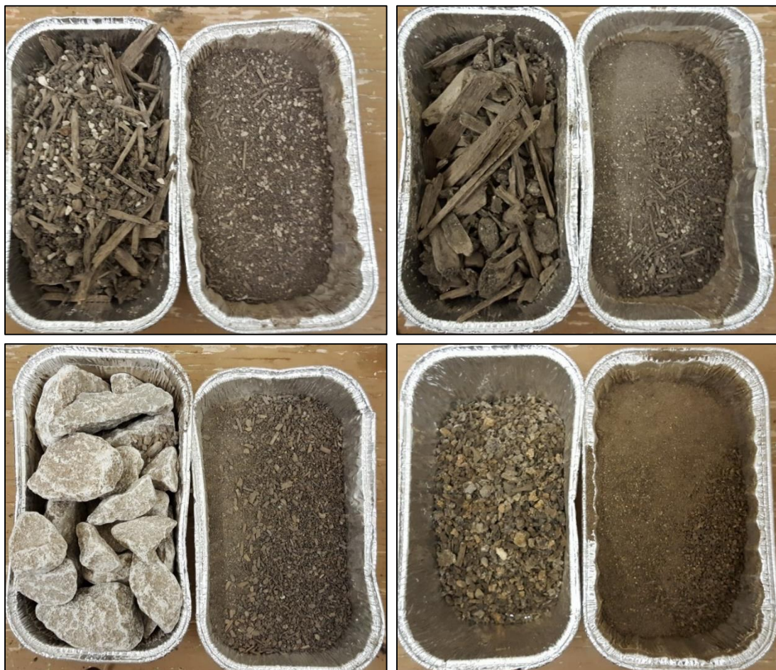
Figure 3-1 Photos of the greater than 2000 \mu\text{m} fraction (left in each photo) and the less than 2000 \mu\text{m} fraction (right in each photo). The less than 2000 \mu\text{m} fraction was used for the hydrometer test. Top row from left to right C3N, C3S. Bottom row from left to right RO, H.
