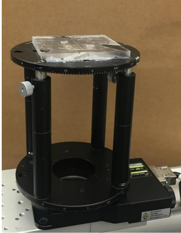
Figure 7.2: Motorized rotation stage (Model SGSP-160YAW, OptoSigma).
