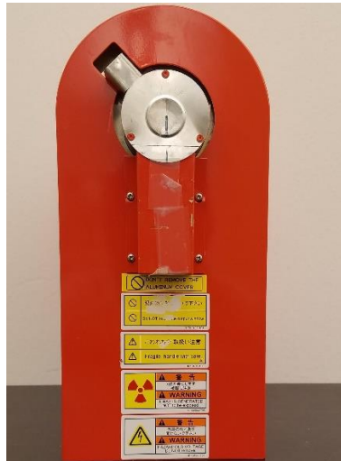
Figure 3.1: X-ray Source (Model L8121-01, Hamamatsu Photonics) used in the prototype.
