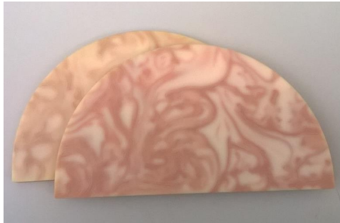
Figure 6.1. Heterogenous phantom mimicking the 70% glandular- 30% adipose breast density. A contrast detail test pattern was embedded to simulate different tumor sizes.
