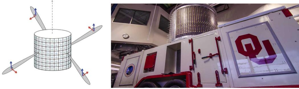
Figure 4.1: CPPAR antenna array and demonstrator designed and fabricated at the University of Oklahoma (From [4]).
