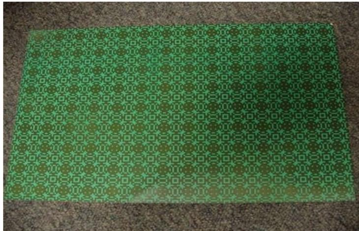
Figure 6.3: A sample design of a dual-band Electromagnetic Bandgap (EBG) Artificial Magnetic Conducting (AMC) ground plane fabricated at the Pennsylvania State University.
