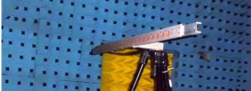
Figure 1.4: 19-element frequency scanning antenna array under test in the Federal Aviations Administration (FAA) anechoic chamber (From [6]).
