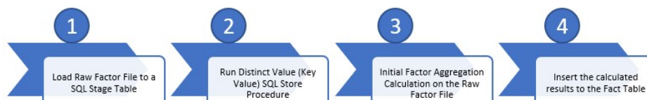
Figure (4.9) Process Steps for an Individual Raw Factor File Process Steps for an Individual Raw Factor File
