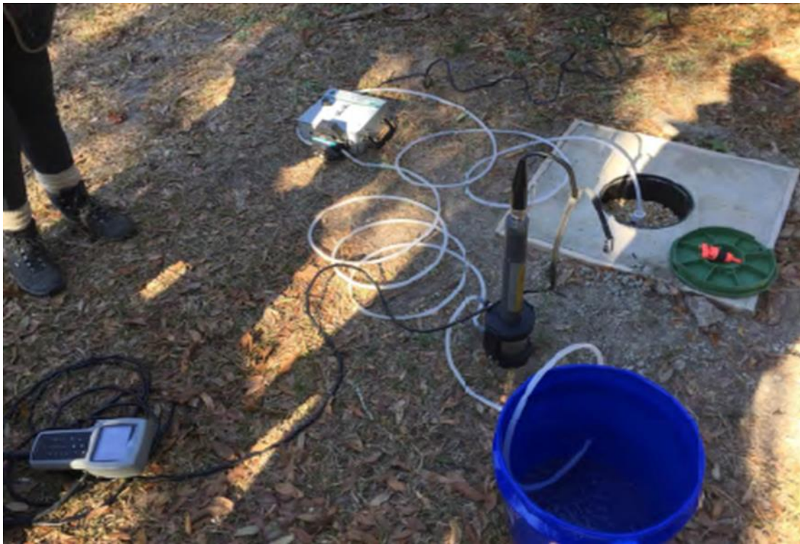
Figure 7: 2016 sampling event employing Peristaltic Pump and YSI 600XL
