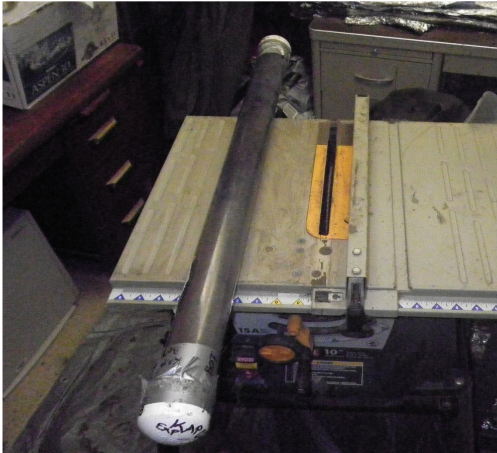
Picture 2. One of the core segments of KAP-01 ready for splitting into two halves; one half as working core and the other archived for reference.
