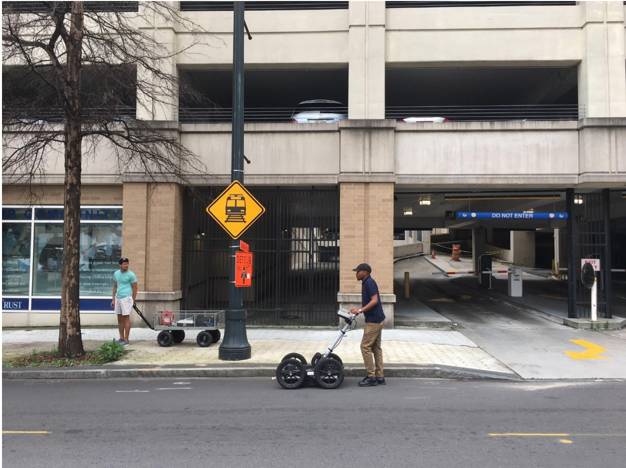
Figure 6: Researcher Fabian Zowam operating the GPR
