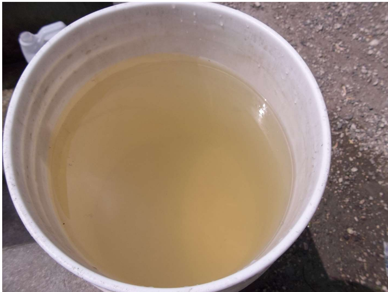
Figure 15: Discoloration of water due to metal pipe usage
