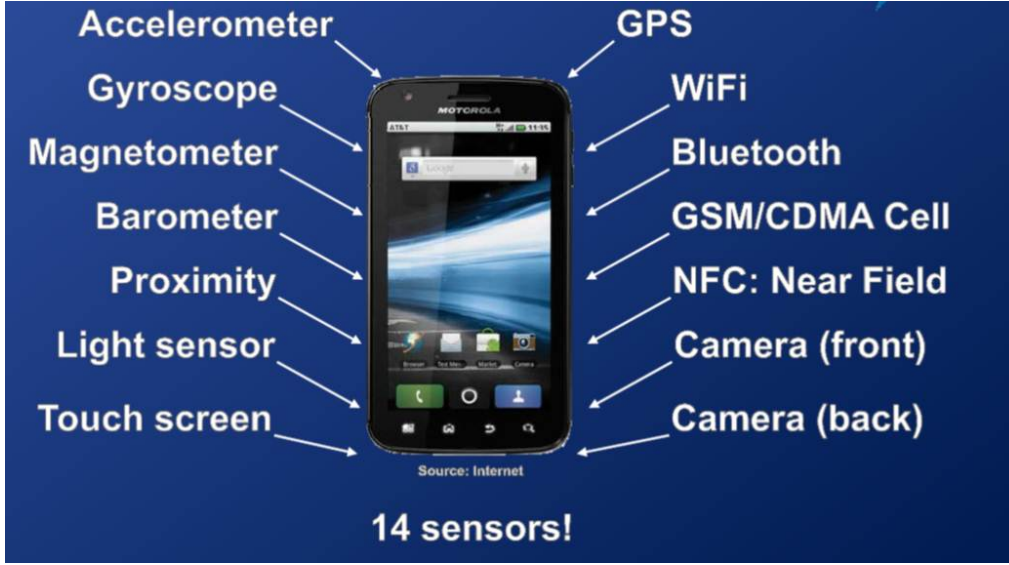
Figure 1.1. Sensors in smartphones
