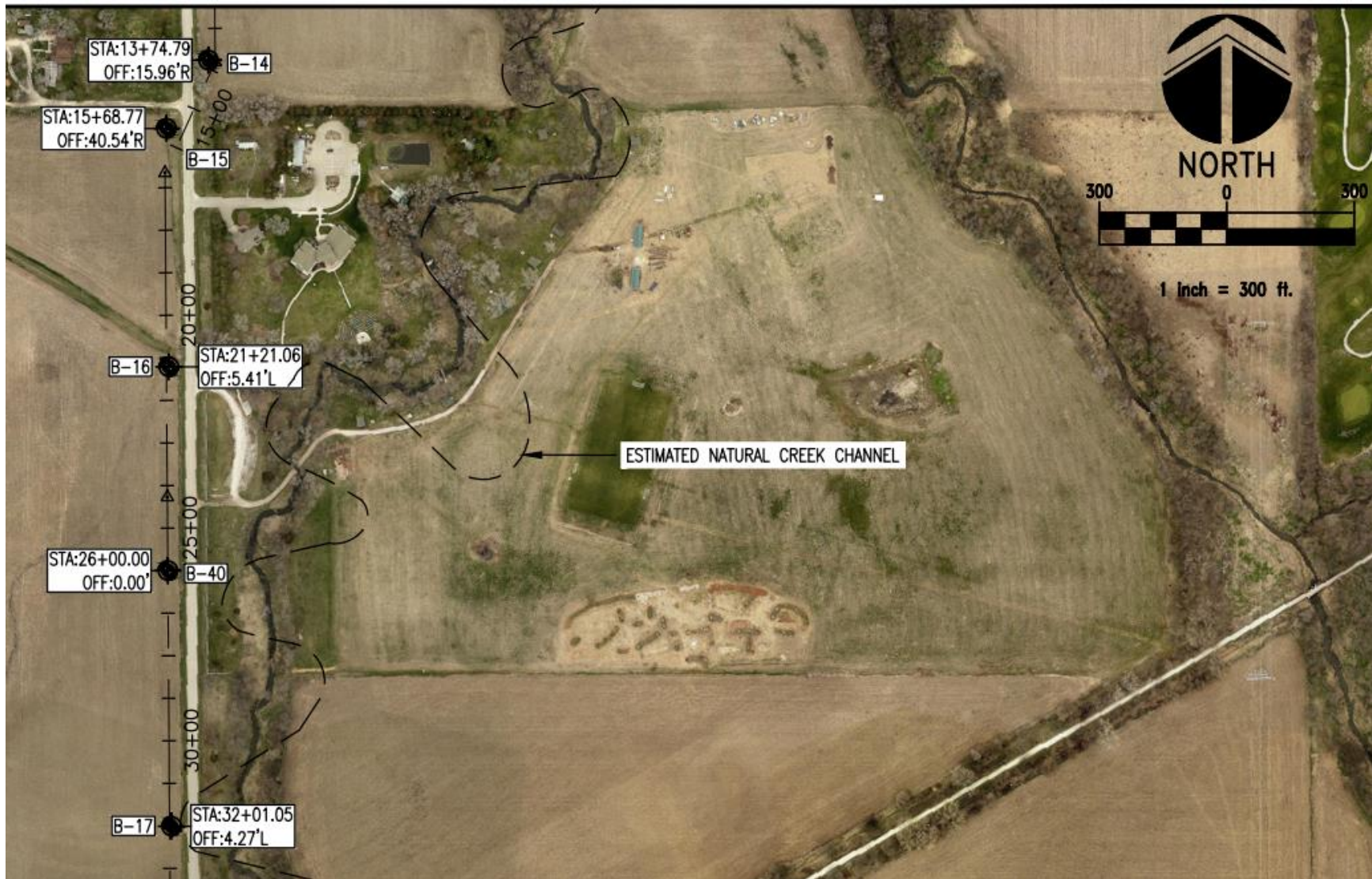
Figure 19: Boring Locations and Estimated Natural Creek Channel from the Sub-Basin E3 Trunk Sewer Report by Schemmer
