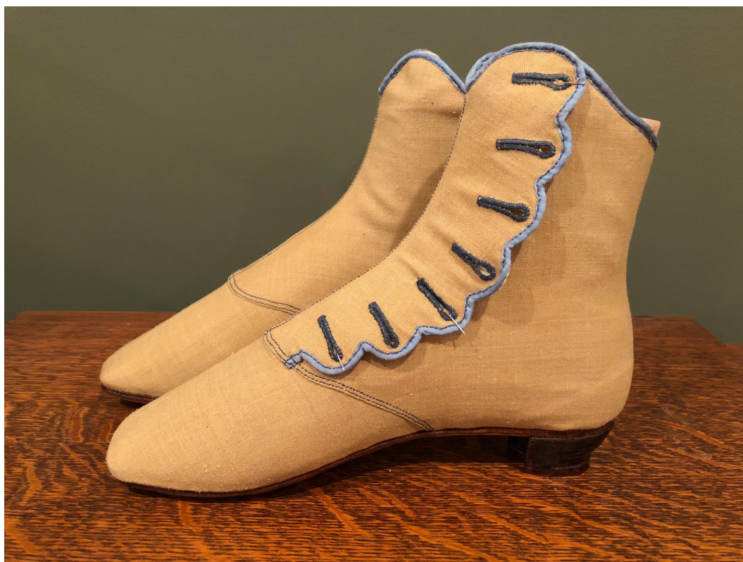
Figure 23: The boots after lasting, cementing, and finishing of the soles and heels. Lasts have not been pulled out yet.
