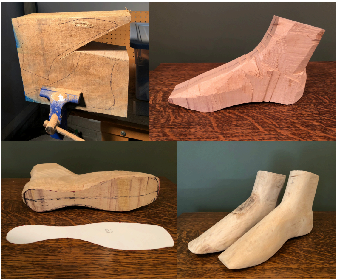
Figure 13: The process of carving a wooden last. Beginning with sawing to shape, carving, planning, then sanding.
