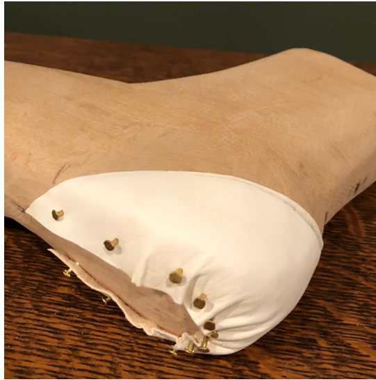
Figure 20: Whittaw heel re-enforcement cut and shaped before inserting.
