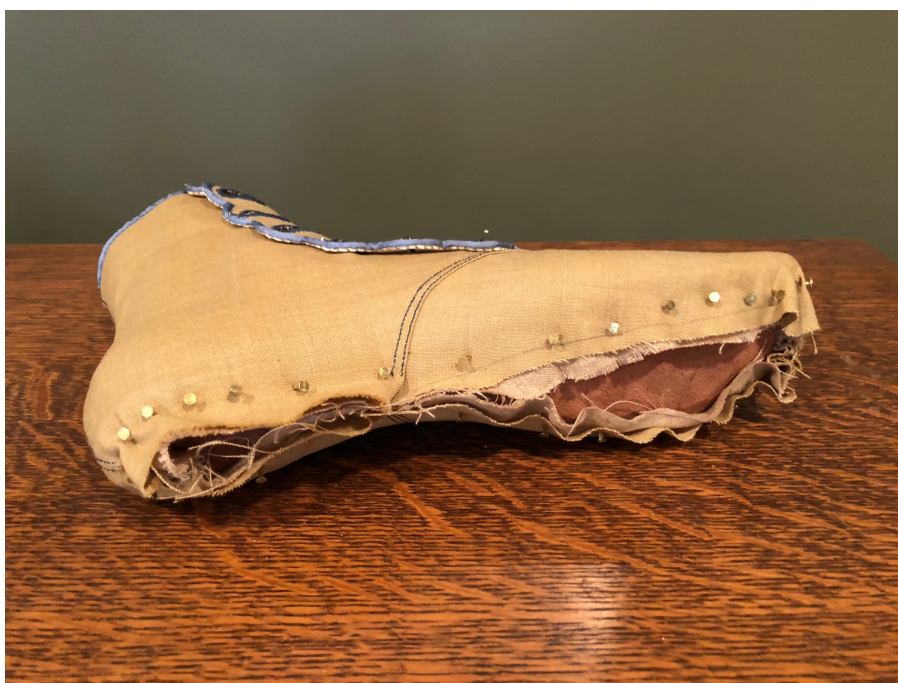
Figure 22: Lasting the uppers over the insole and tacking to hold them in place before cementing.
