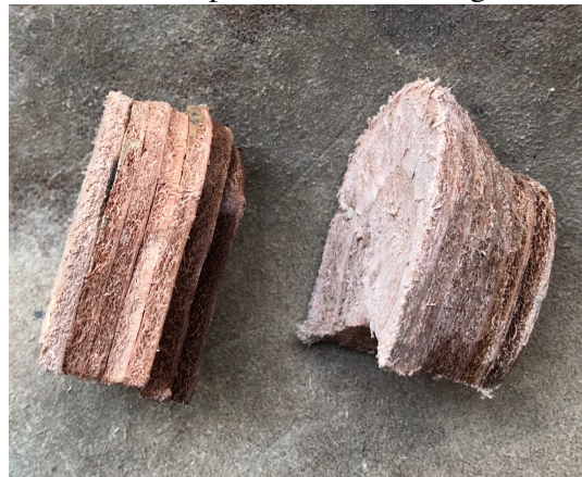
Figure 21: Stacked leather heels cemented and pegged together (left) and carved to shape (right).
