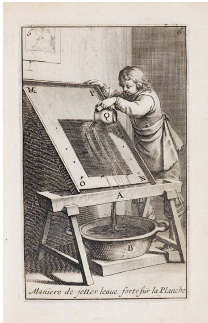
Abraham Bosse (1604-c. 1676), Pouring acid to etch a plate on a slanted board (On the Manner of Etching with Acid and with a Burin, and of Dark-Manner Engraving) , etching, drypoint, and roulette, 1645. Rhode Island School of Design, Gift of Mrs. Herbert N. Straus, 51.004
