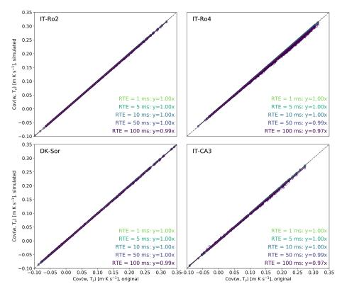
Figure 4. Simulation of RTEs. Covariances w- $T_s$  obtained with a set of simulated random errors of different amplitudes (y axes) are compared to the covariances w- $T_s$  computed with the original time series (x axes), for the four sites. All regressions had an offset equal to zero and  $r^2 > 0.99$ .
