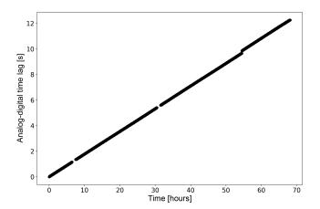
**Figure 9.** Evolution of time lags between two replicates of the same variable (u wind component, but identical results were obtained with v and w), one collected with the SAT native digital format and one collected via analog outputs from the SAT. Data were collected in two files roughly 70 h long and then split into 30 min chunks for the computation of time lags.
