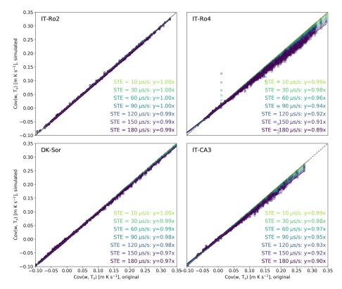
**Figure 5.** Simulation of STE. Covariances w- $T_{\rm S}$  obtained with a set of simulated systematic errors of different amplitudes (y axes) are compared to the covariances w- $T_{\rm S}$  computed with the original time series (x axes), for the four sites. All regressions had an offset equal to zero and  $r^2 > 0.98$ .
