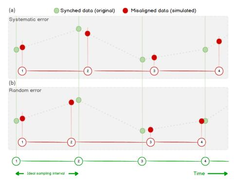
Figure 3. Sketch of the timing error simulation via linear interpolation. Green dots represent original  $T_s$  data points, equally spaced at the prescribed (nominal) time steps. In (b), RTEs are simulated as time steps randomly varying around the nominal value. In (a), STEs are simulated as a time step larger than the nominal one, whereby the difference between the assigned and correct timestamps always increase in time.
