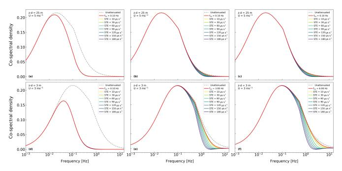
Figure 7. Effect of adding artificial STEs to three EC systems characterized by different cutoff frequencies (0.1, 3.0, and 6.0 Hz for d, e, and f, respectively) and by different measurement height and mean wind speed (from a-c to d-f).
