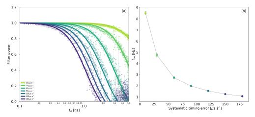
**Figure 6.** Transfer function for the STE at different error amounts, as derived using Eqs. (2) and (3), using data from site IT-CA3 (a). Mean values and  $3.5\sigma$  ranges of the transfer function cutoff frequencies across the fours sites, as a function of the error amount (b).
