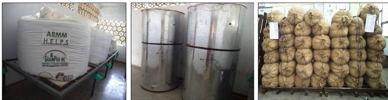
Figure 2. Experimental setup of hermetic bags, metallic bins, and gunny bag piles after the sensors were installed. Hermetic bags were mounted on stands with anti-rodent devices.
