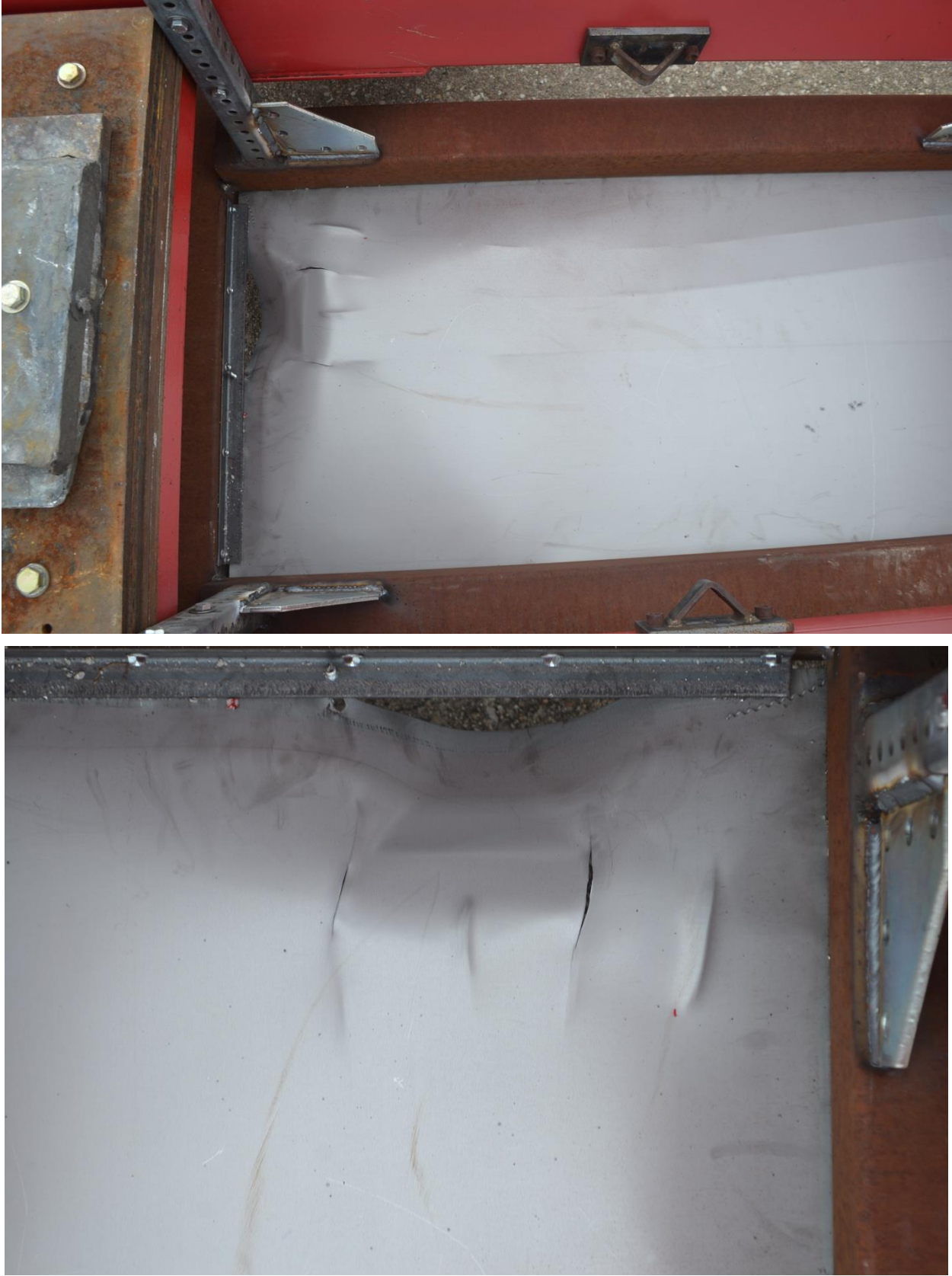
Figure 25. Simulated Floorpan Damage, Test No. MWFPF-1
