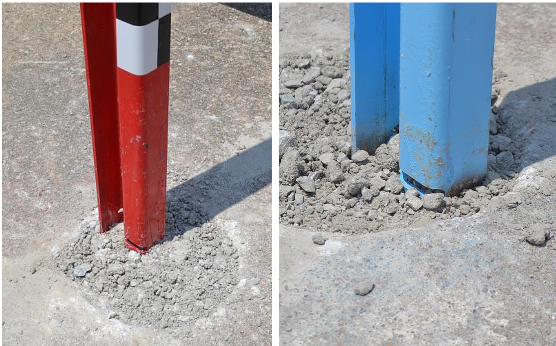
Figure 54. MWP with \frac{3}{8} -in. x 1\frac{1}{8} -in. (10-mm x 29-mm) Weakening Slots
