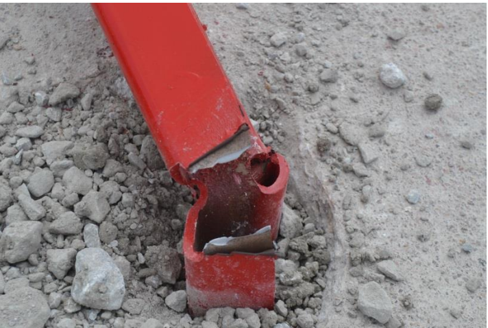
Figure 88. Time-Sequential and Post-Impact Photographs, Test No. MWFPF-17 Post 1
