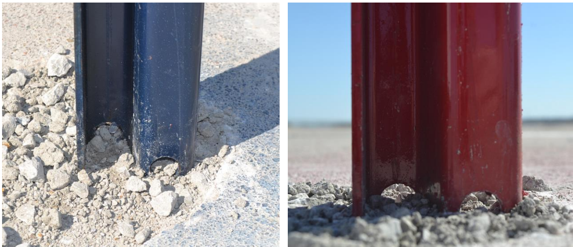
Figure 31. MWP with ¾-in. (19-mm) Diameter Weakening Holes
