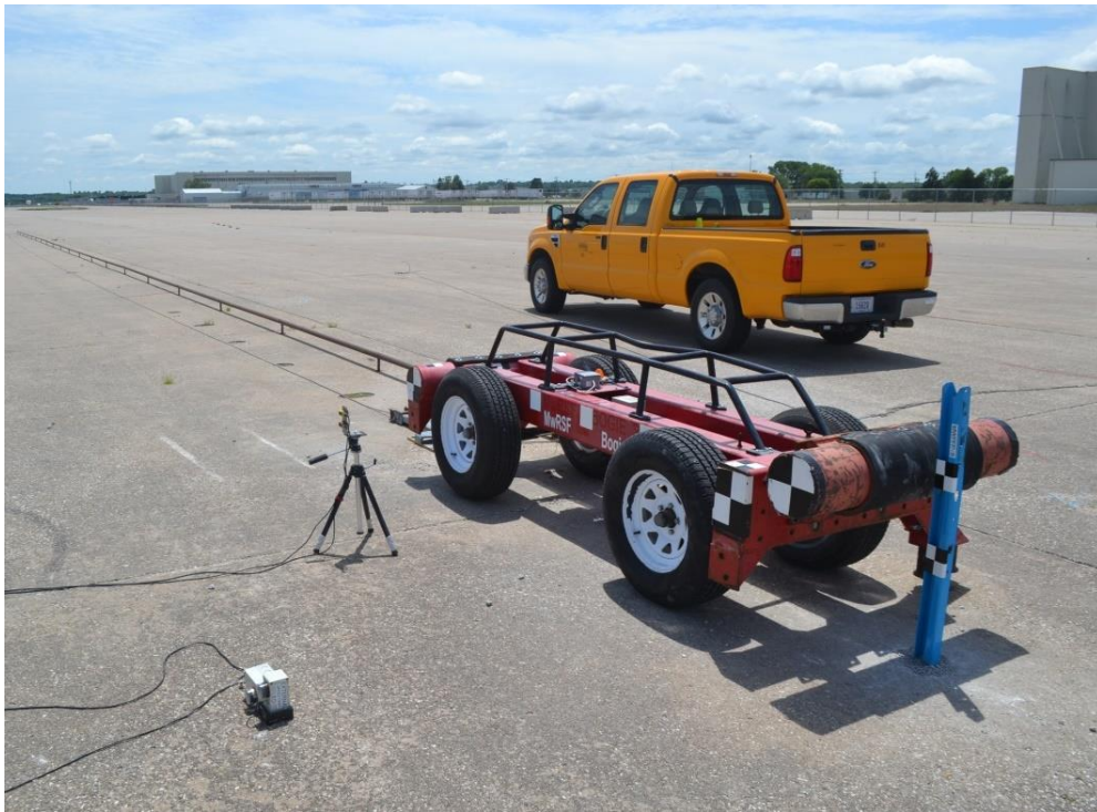
Figure 78. Second Rigid-Frame Bogie and Guidance Track
