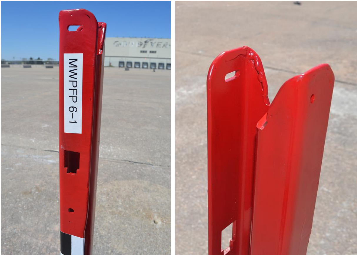
Figure 41. MWP with Simulated No. 1 Edge Rounding, Test No. MWPFPP-6
