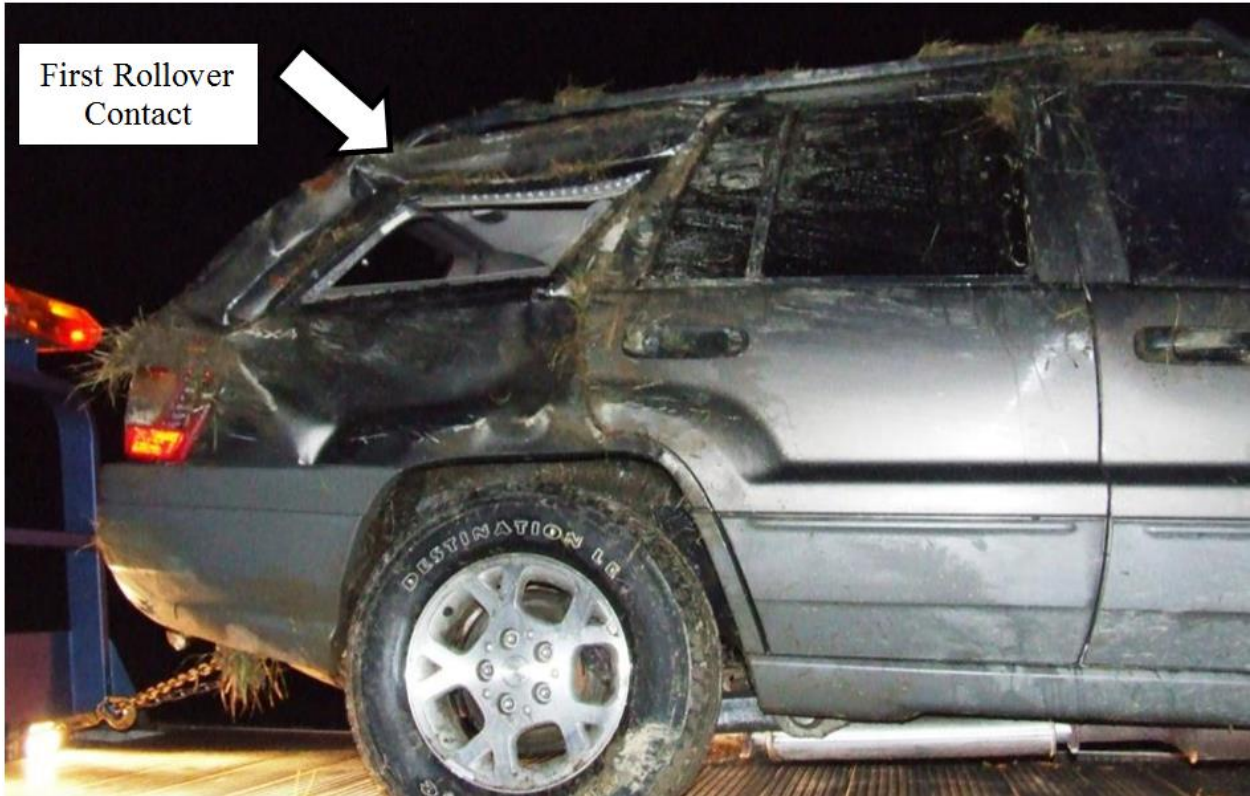
Figure 134. Example Rollover Crash Caused by High Orientation Angle at Impact
