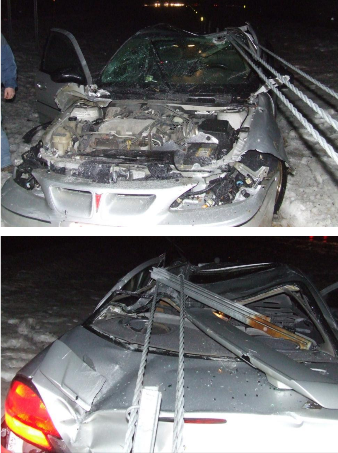
Figure 92. Potential Penetration Crash on Nucor NU-CABLE Barrier
