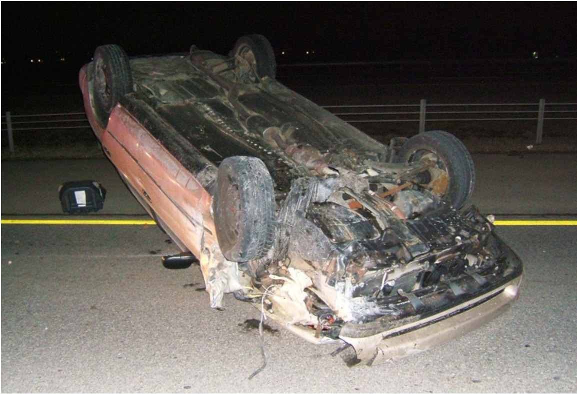
Figure 137. Example of Post Snag Rollover Crash
