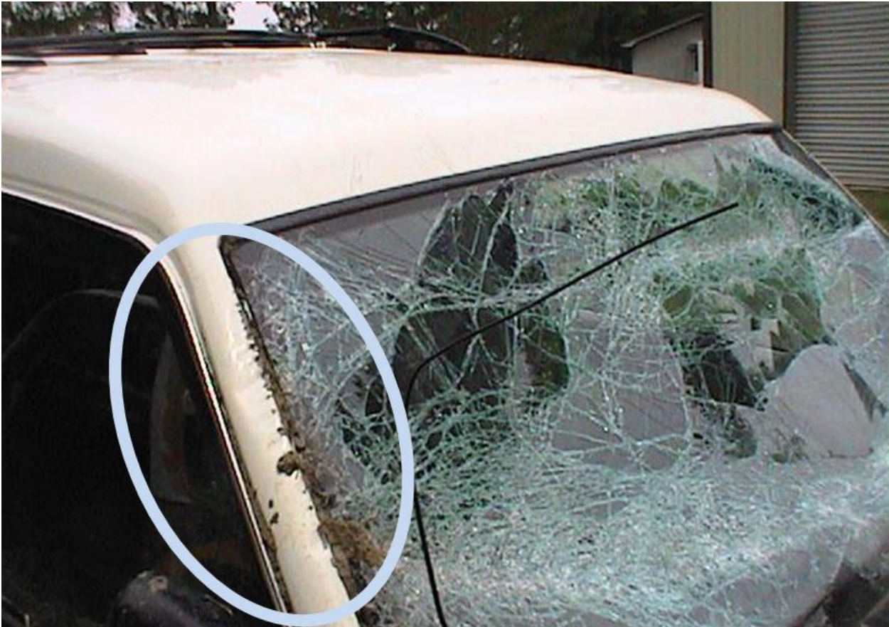
Figure 106. Brush Guard Prying Penetration with Cable Contact Striations on A-Pillar
