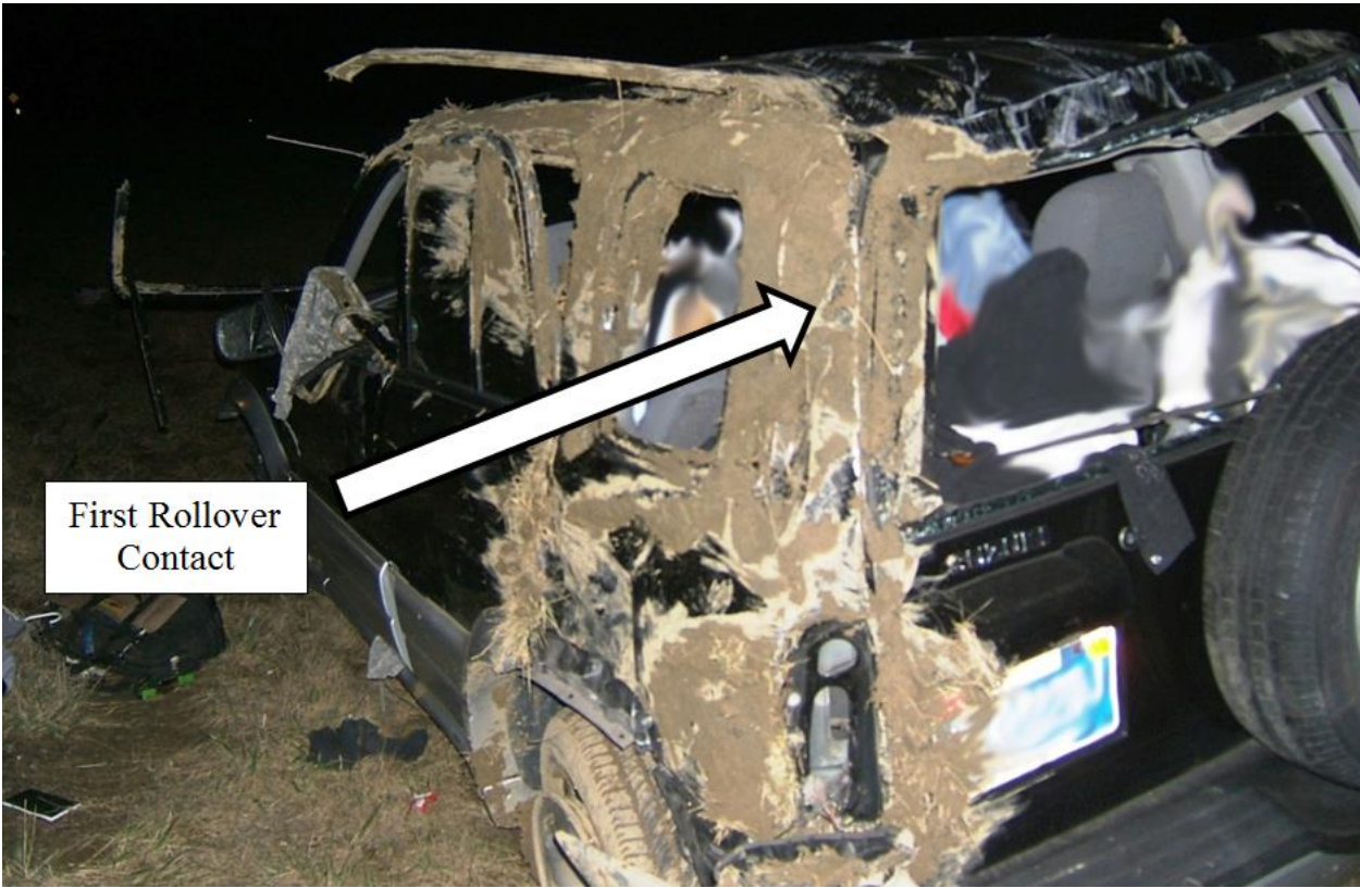
Figure 135. Second Example Rollover Crash Caused by High Orientation Angle at Impact
