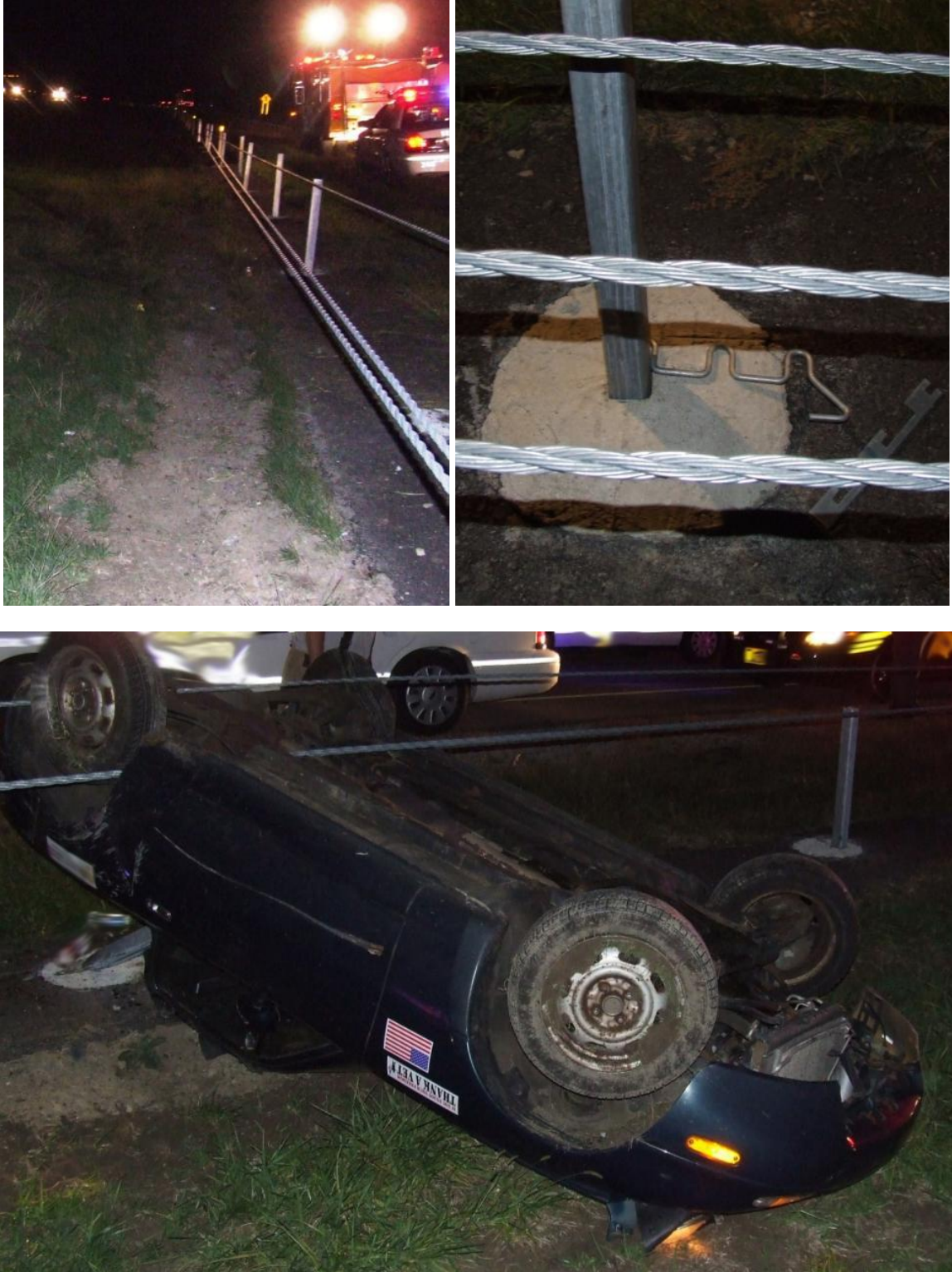
Figure 138. Example of Post Snag Rollover Crash
