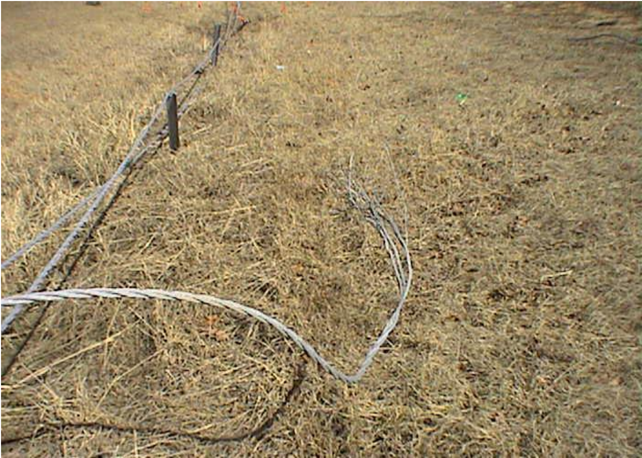
Figure 107. Splice Failure Penetration
