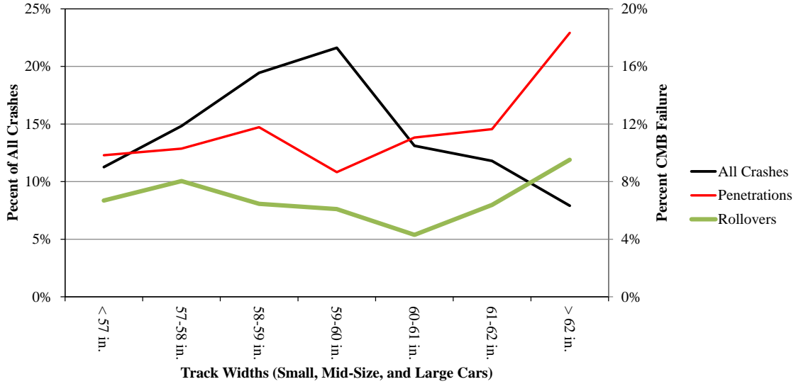
Figure 31. Crash Result Based on Track Width, Small, Mid-Size, and Large Cars
