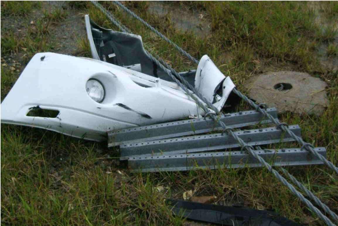
Figure 89. Override Penetration Crash Vehicle Final Position and Removed Bumper Cover
