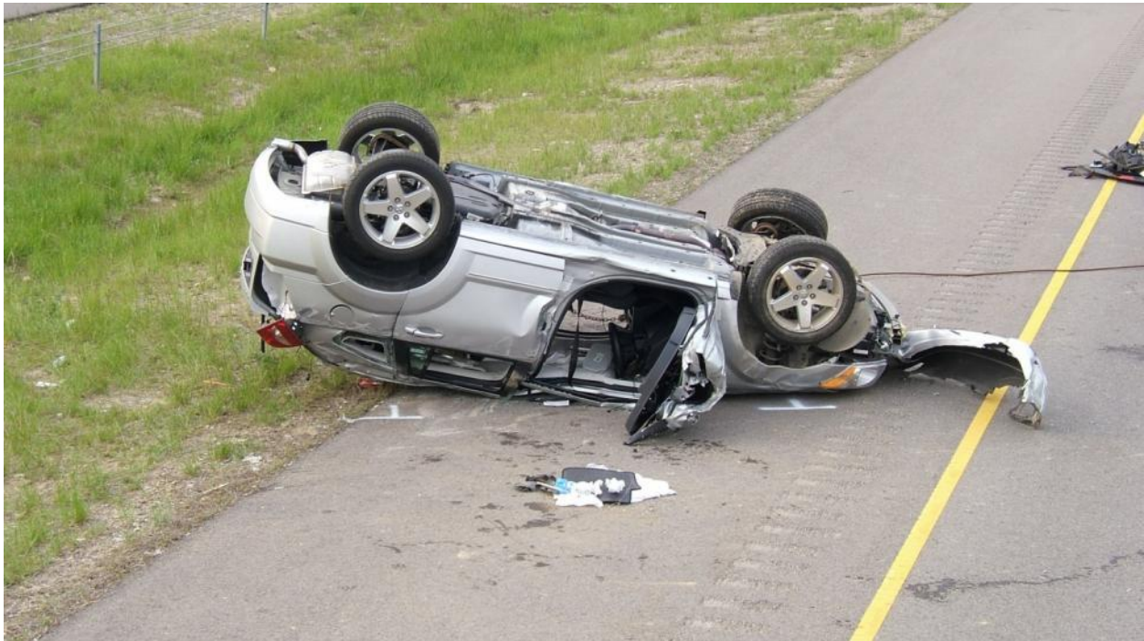
Figure 131. Example Rollover Crash Caused by High Redirection on Back Slope
