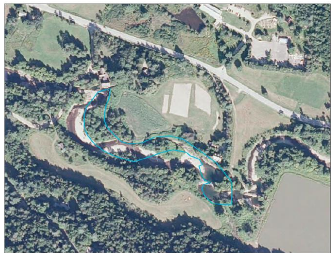
Figure 3.2: Channelization of Mad River in Waitsfield, VT, showing change in river pathway in blue from 1973 – 2004.
