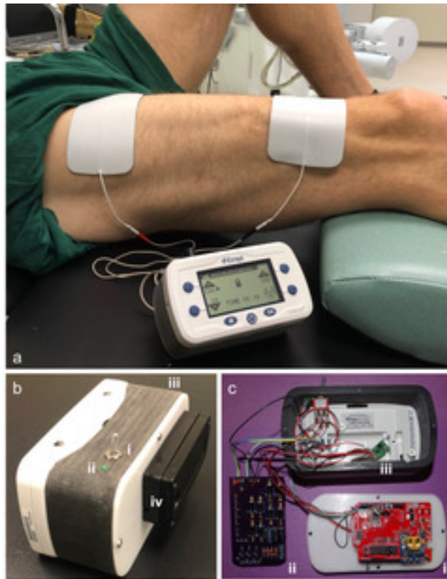
Figure 3.2: Smart EMPI system can track the duration, intensity, and timing of NMES rehabilitation sessions (a). System is composed of an Arduino (c-iii) and custom circuitry for quantifying device usage (c-ii), and is integrated within a 3D printed enclosure secured to the back of the EMPI (b-iv). Power is provided by two AA batteries secured in an external housing (b-i) and is controlled by a master switch (b-ii) and step-up regulator (c-i). An external LED (b-iii) indicates when the batteries need to be replaced.
