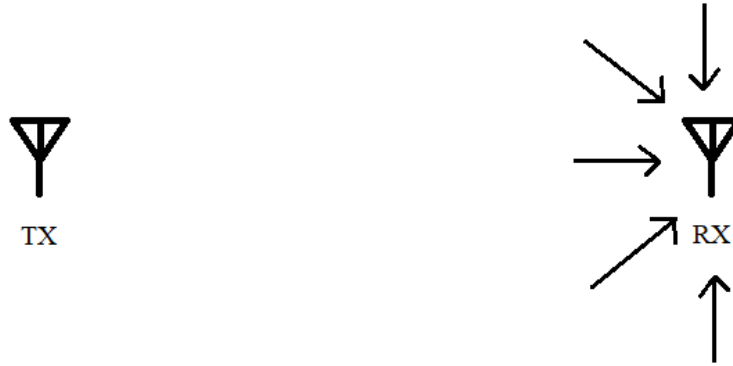
Figure 2.2: A sketch of a Rayleigh communication channel. The dominant LOS component is no longer discernible from the multipath components.
