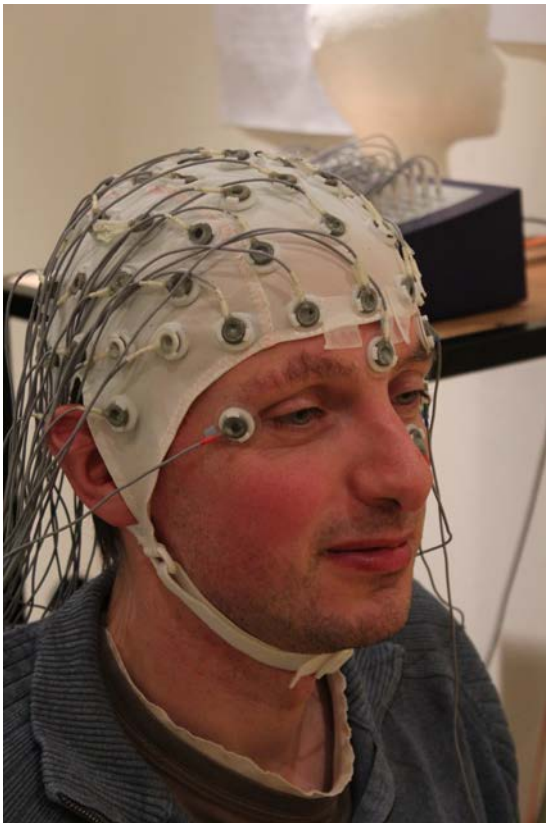
Figure 9. A typical EEG cap setup on a human subject. Photo by Chris Hope. Permission to republish granted to Tim Sheerman-Chase. ( https://commons.wikimedia.org/wiki/File:Three_quarter_view_of_EEG_subject.jpg , „Three quarter view of EEG subject“, https://creativecommons.org/licenses/by/2.0/legalcode
