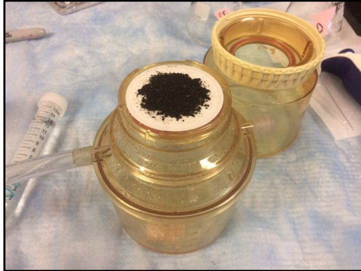
Figure 4: Filter setup for sulfate flow through experiment. An open top soil packet is seen resting on the bottom section (effluent collection) of a Nalgene filter pod.
