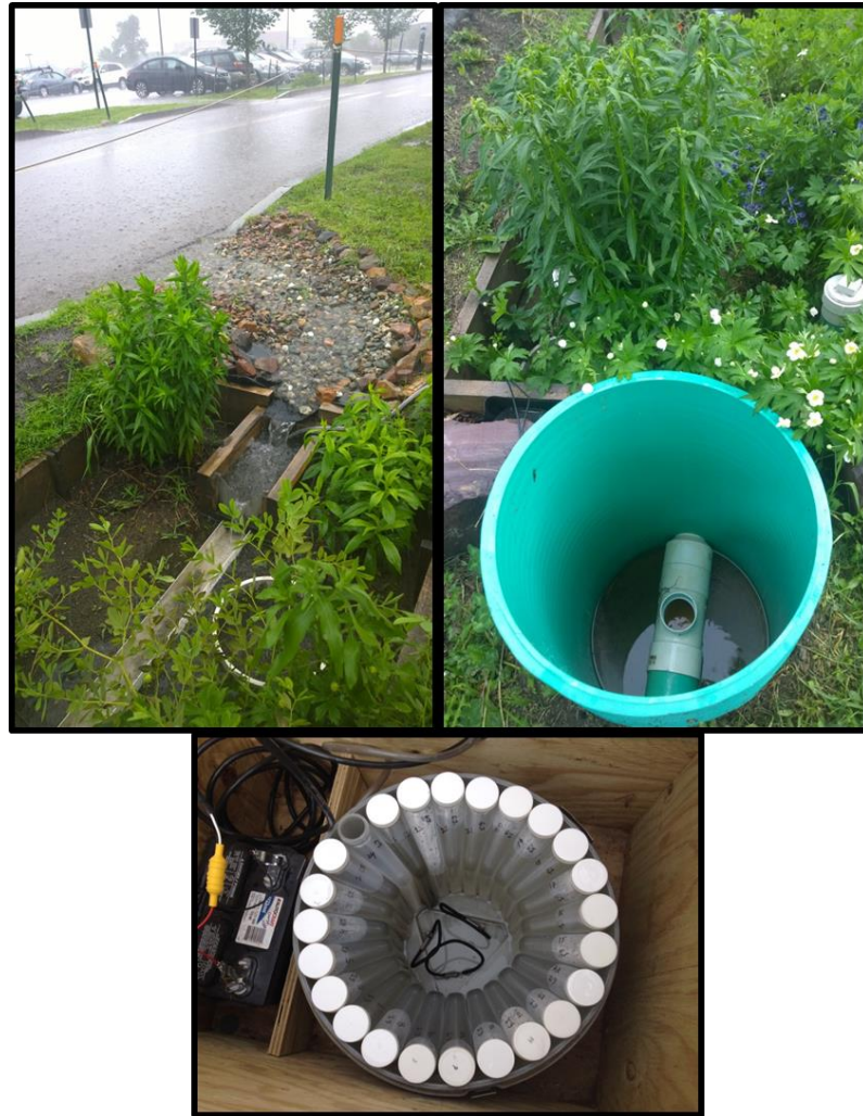
Fig. 2. (Top left, Top Right, Bottom): Road runoff being conveyed via curb cut and rock-line swale into the v-notch weir where influent water is sampled, effluent water sampling location from an underdrain pipe 4ft deep belowground, stormwater samples collected in up to 24 bottles in the autosampler.
