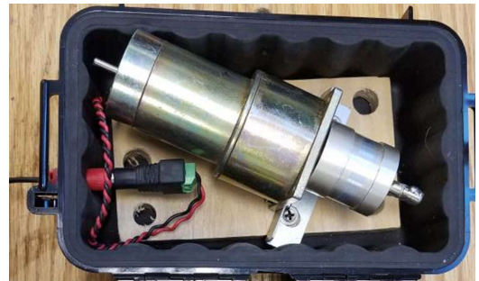
Figure 55 (a) moisture sensor in soil, and (b) rotating magnet source before being buried under concrete slab
