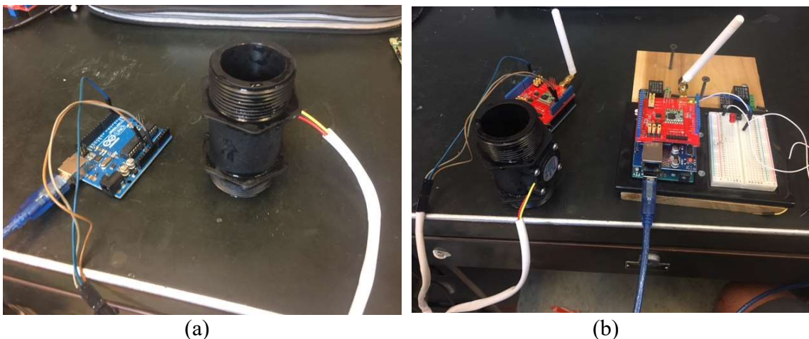
Figure 50 (a) Commercial flow meter connected to Arduino for data collection, and (b) shown connected to LoRa transceiver components
