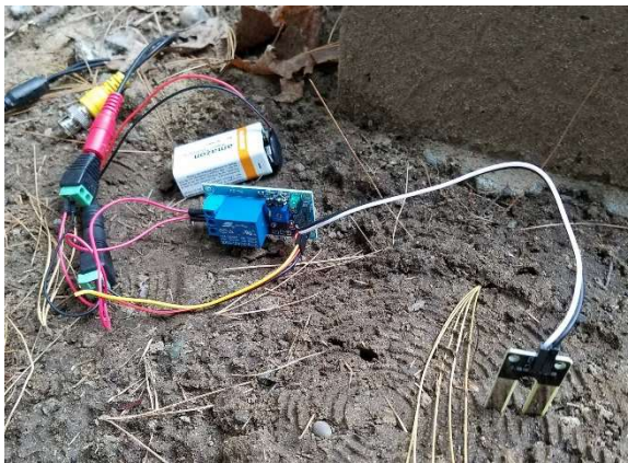
Figure 55 (a) moisture sensor in soil, and (b) rotating magnet source before being buried under concrete slab
