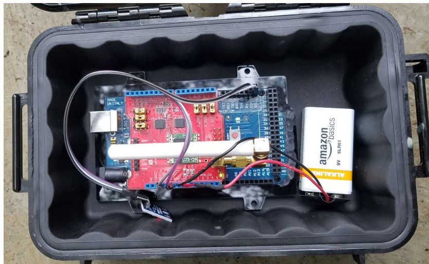
Figure 48 Magnetometer receiver (Arduino Mega with HMC5883L magnetometer) with LoRa transmitter in weatherproof case
