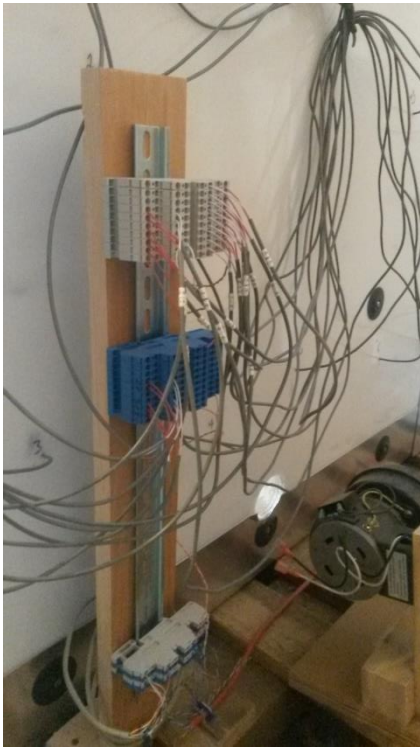
Figure 7: 1-Wire Bus Terminal
