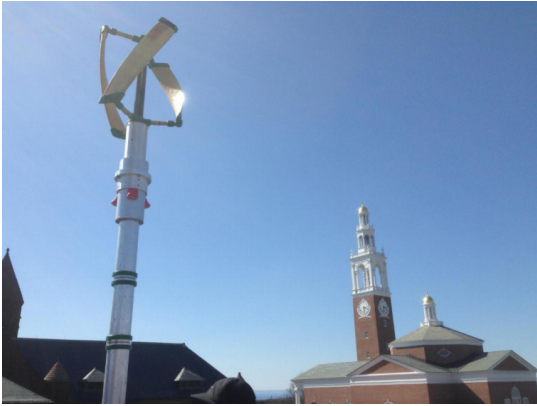
Figure 1: VAWT with Bamboo Blades Built and Designed at the University of Vermont
