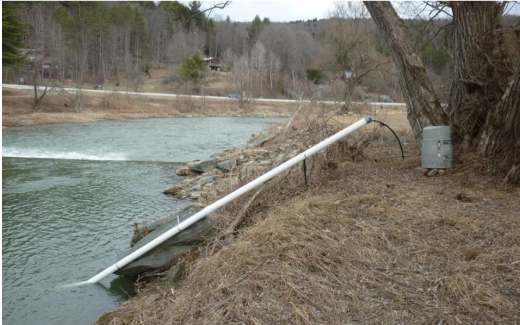
Mad River turbidity sensor installation looking downstream. USGS gauge on opposite bank
