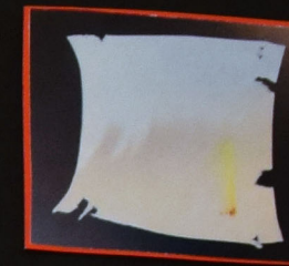
2D chromatography using acetone under light
